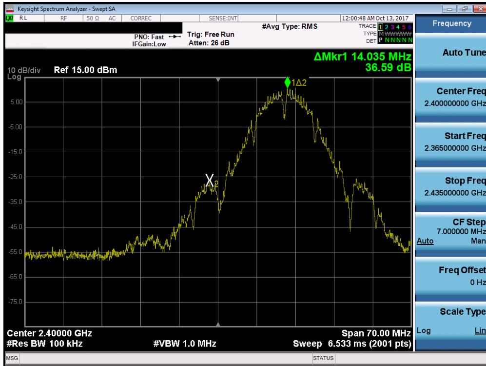
Plot 7-43. Band Edge Plot (802.11b – Ch. 1)
