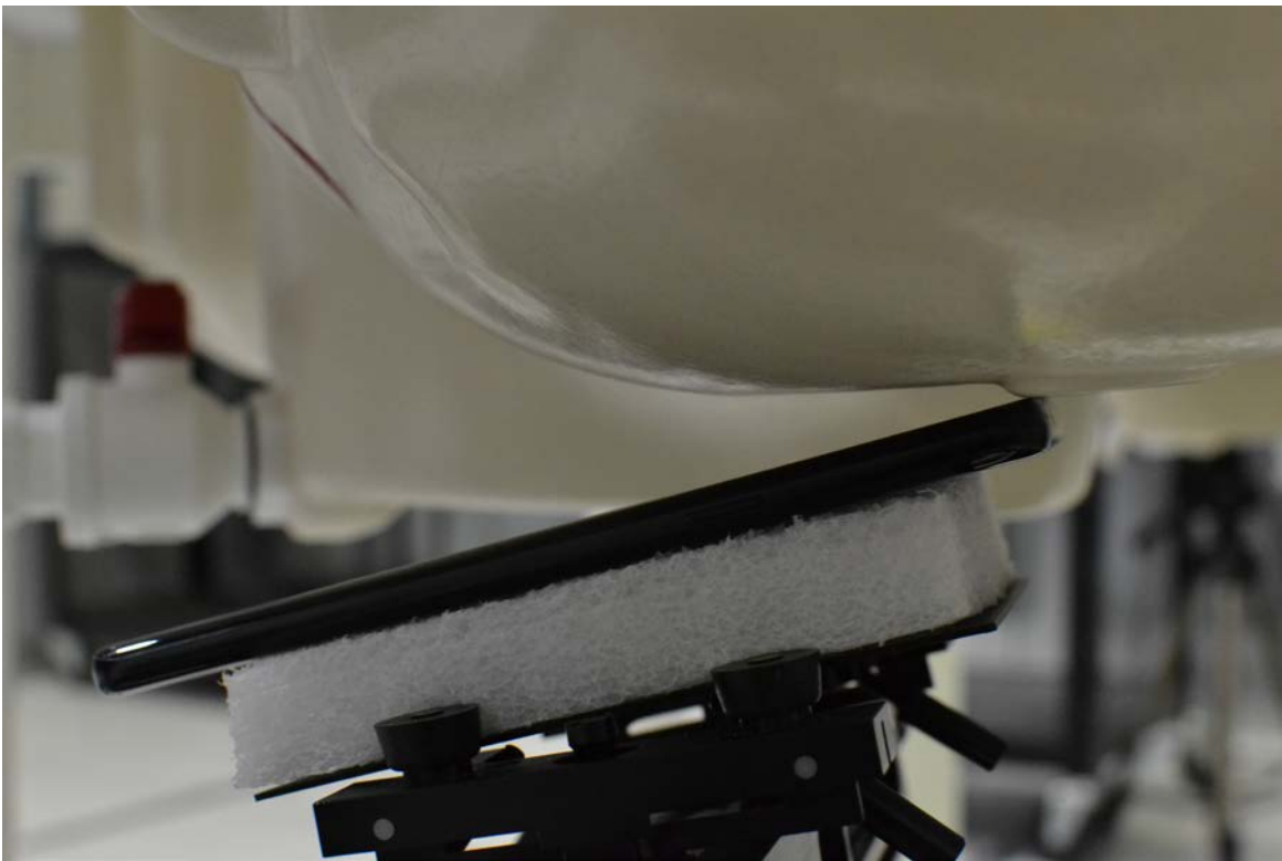
SAR Test Setup Photo 4 – Left Tilt
