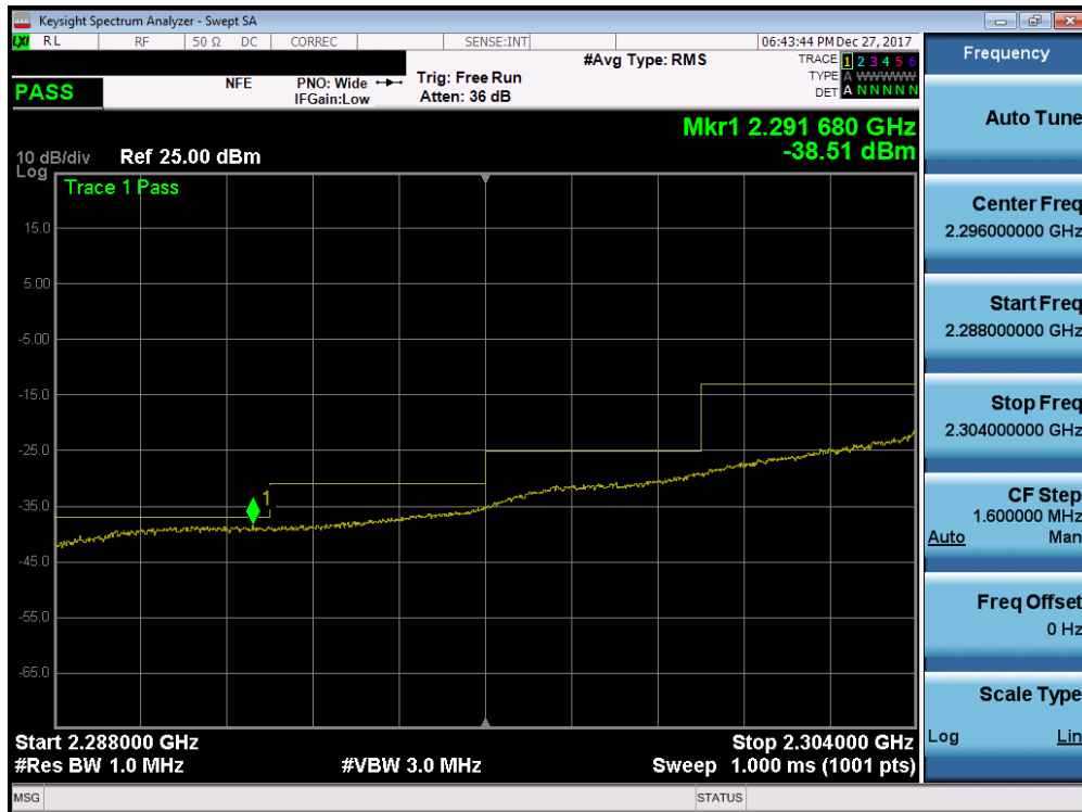
Plot 7-6. Lower Extended Band Edge Plot (Band 30 - 10.0MHz QPSK - Full RB Configuration- Antenna B)
