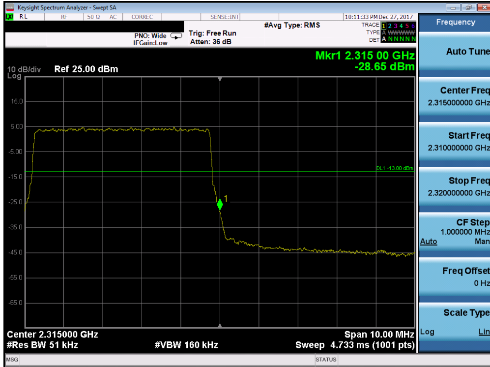
Plot 7-11. Upper Band Edge Plot (Band 30 - 5.0MHz QPSK - Full RB Configuration- Antenna A)
