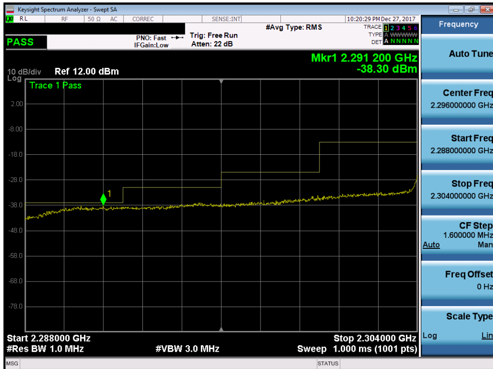
Plot 7-14. Lower Extended Band Edge Plot (Band 30 - 10.0MHz QPSK - Full RB Configuration- Antenna A)
