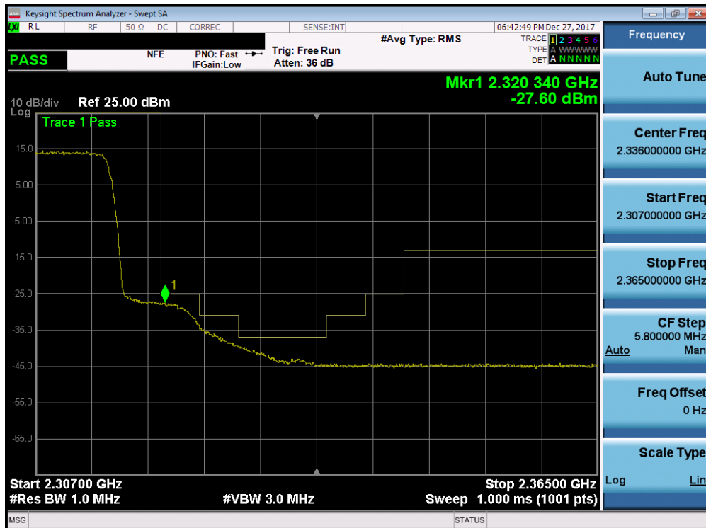
Plot 7-8. Upper Extended Band Edge Plot (Band 30 - 10.0MHz QPSK - Full RB Configuration- Antenna B)
