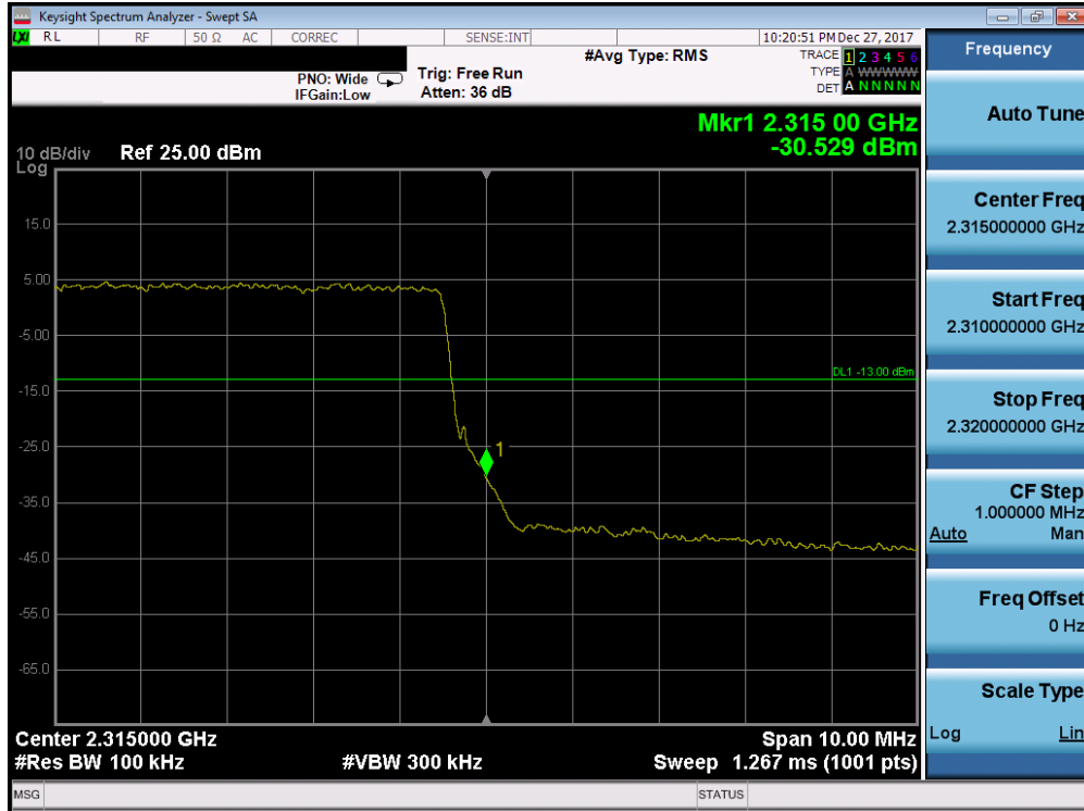
Plot 7-15. Upper Band Edge Plot (Band 30 - 10.0MHz QPSK - Full RB Configuration- Antenna A)
