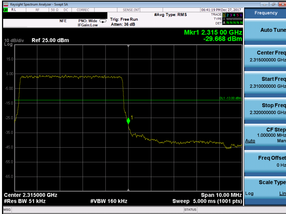
Plot 7-3. Upper Band Edge Plot (Band 30 - 5.0MHz QPSK - Full RB Configuration- Antenna B)
