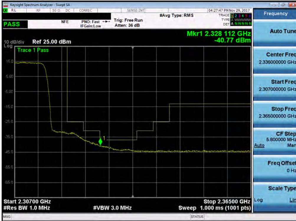
Plot 7-354. Upper Extended Band Edge Plot (Band 30 - 10.0MHz QPSK - Full RB Configuration- Antenna A)
