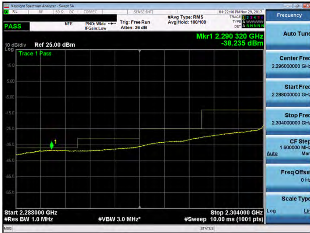
Plot 7-352. Lower Extended Band Edge Plot (Band 30 - 10.0MHz QPSK - Full RB Configuration- Antenna A)
