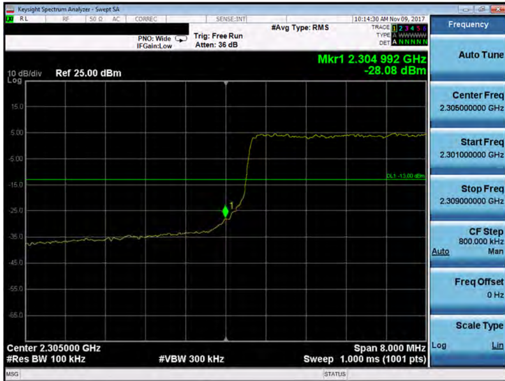
Plot 7-342. Lower Band Edge Plot (Band 30 - 10.0MHz QPSK - Full RB Configuration- Antenna B)
