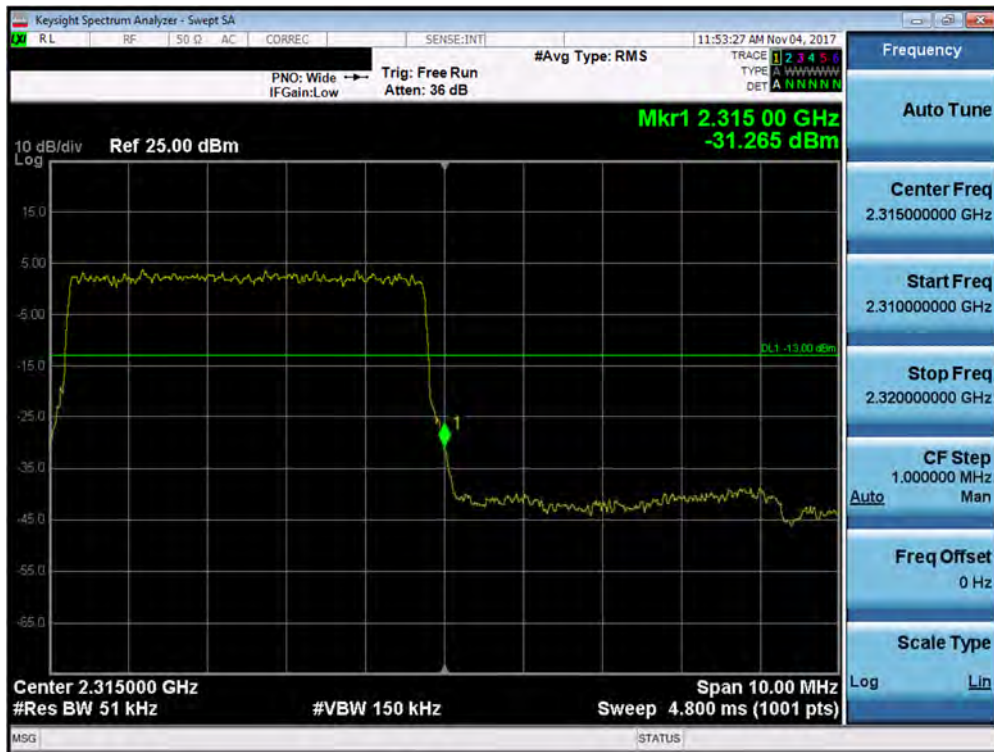
Plot 7-340. Upper Band Edge Plot (Band 30 - 5.0MHz QPSK - Full RB Configuration- Antenna B)
