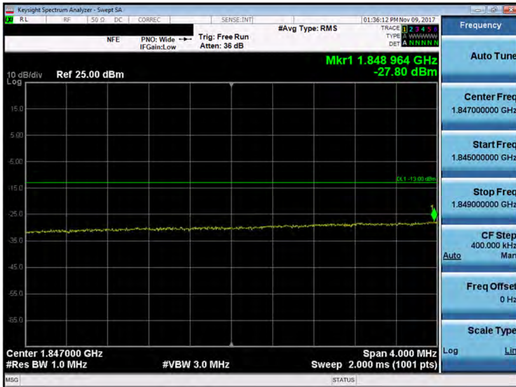
Plot 7-326. Lower Extended Band Edge Plot (Band 2/25 - 15.0MHz QPSK - Full RB Configuration)
