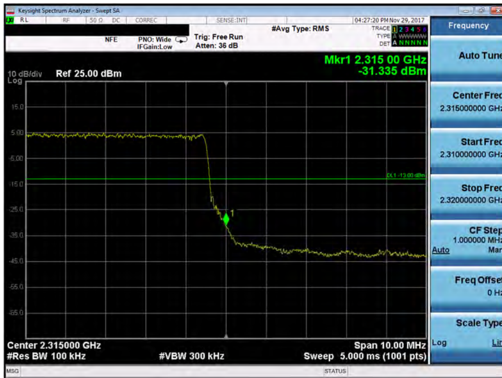
Plot 7-353. Upper Band Edge Plot (Band 30 - 10.0MHz QPSK - Full RB Configuration- Antenna A)
