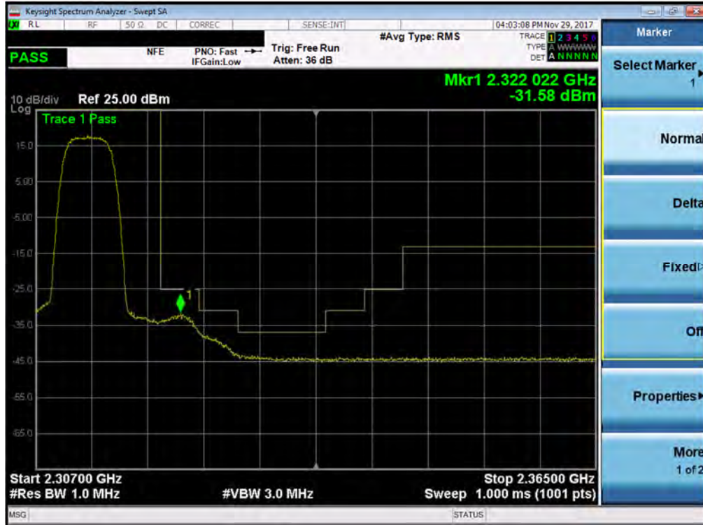
Plot 7-350. Upper Extended Band Edge Plot (Band 30 - 5.0MHz QPSK - Full RB Configuration- Antenna A)
