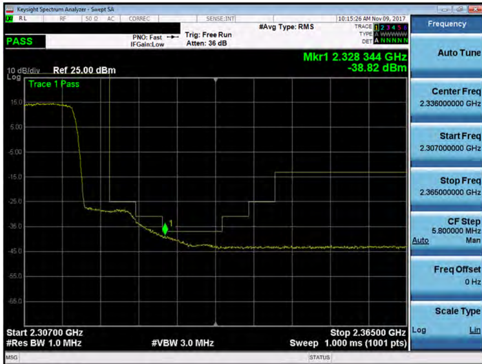
Plot 7-345. Upper Extended Band Edge Plot (Band 30 - 10.0MHz QPSK - Full RB Configuration- Antenna B)
