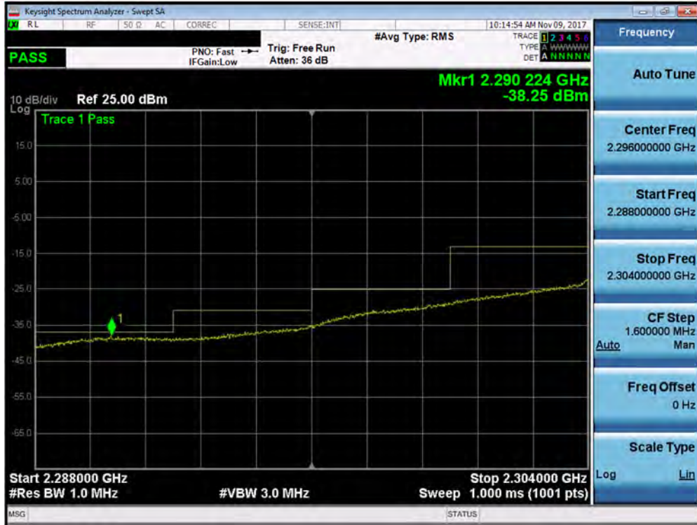
Plot 7-343. Lower Extended Band Edge Plot (Band 30 - 10.0MHz QPSK - Full RB Configuration- Antenna B)
