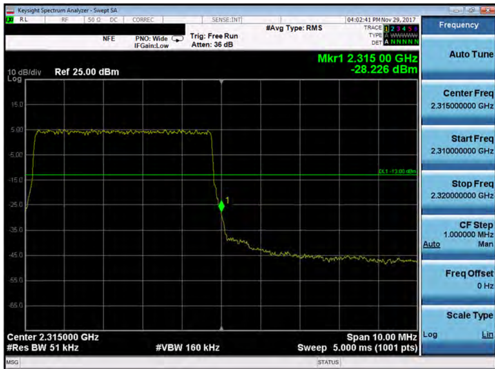
Plot 7-349. Upper Band Edge Plot (Band 30 - 5.0MHz QPSK - Full RB Configuration- Antenna A)
