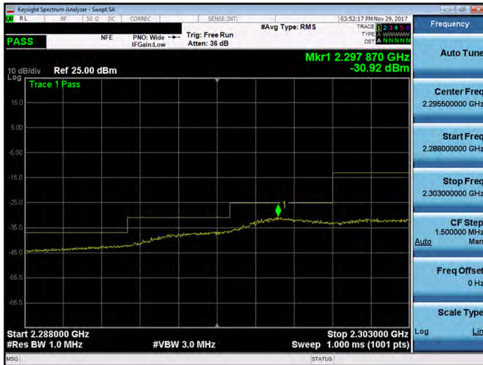
Plot 7-347. Lower Extended Band Edge Plot (Band 30 - 5.0MHz QPSK - Full RB Configuration - Antenna A)
