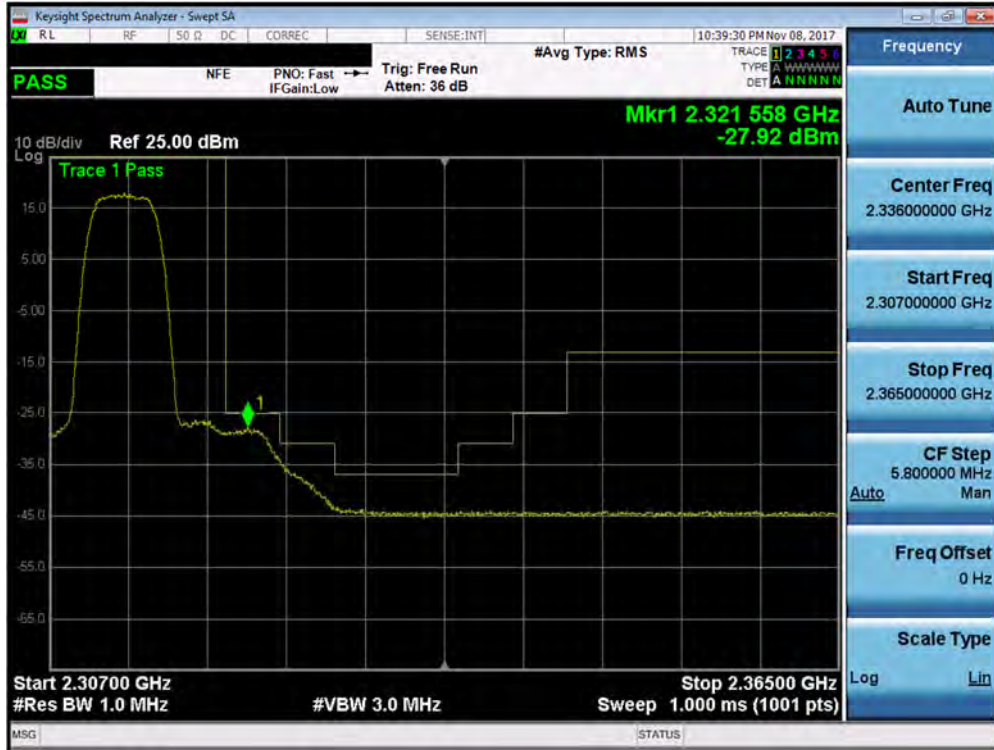
Plot 7-341. Upper Extended Band Edge Plot (Band 30 - 5.0MHz QPSK - Full RB Configuration- Antenna B)
