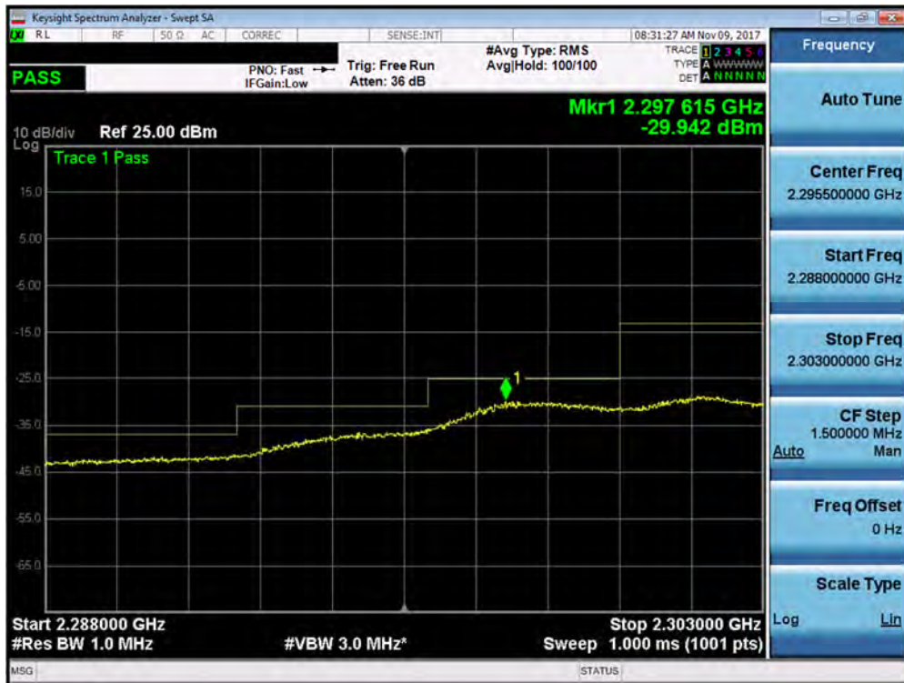
Plot 7-338. Lower Extended Band Edge Plot (Band 30 - 5.0MHz QPSK - Full RB Configuration – Antenna B)
