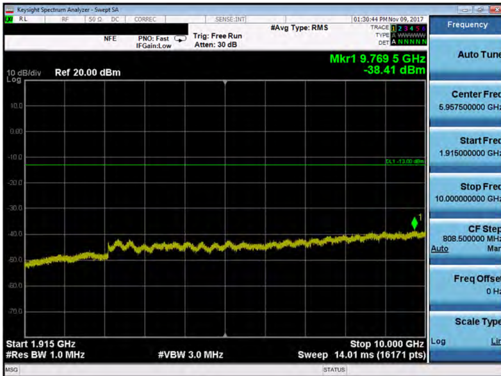
Plot 7-176. Conducted Spurious Plot (Band 2/25 - 10.0MHz QPSK - RB Size 1, RB Offset 0 - Low Channel)
