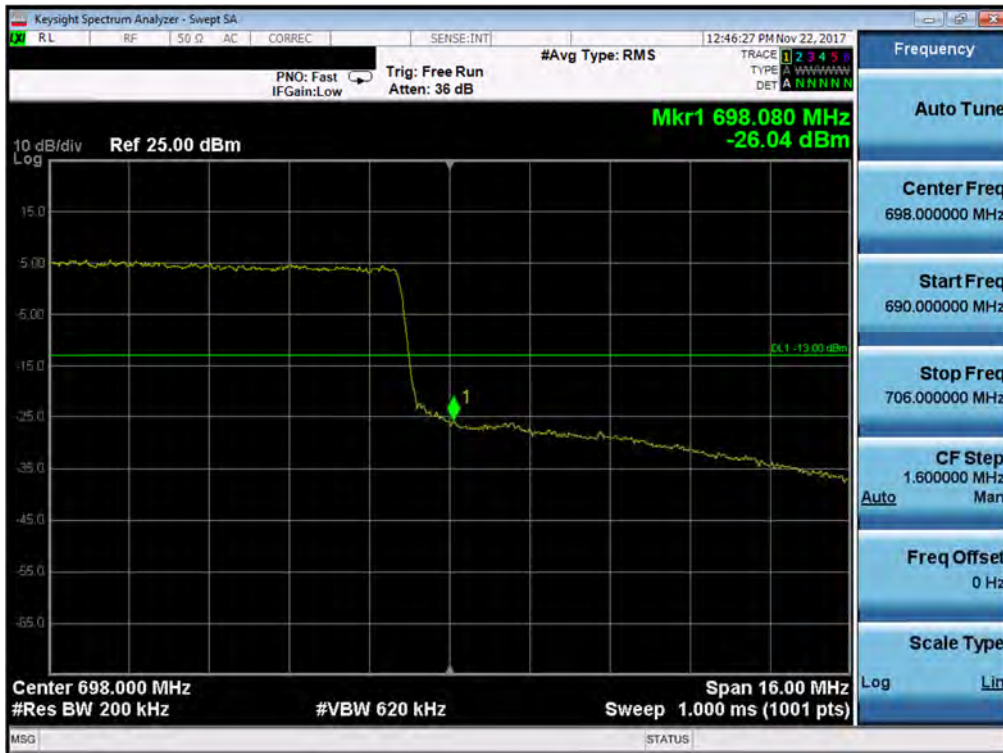
Plot 7-236. Upper Band Edge Plot (Band 71 - 20.0MHz QPSK - Full RB Configuration)
