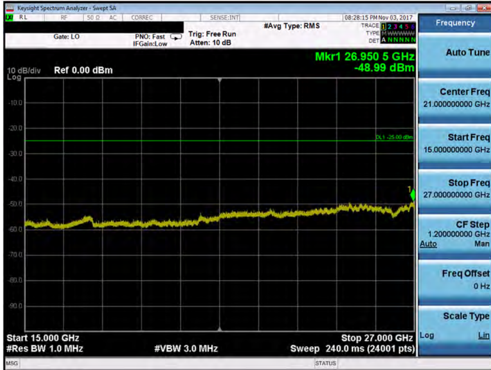
Plot 7-228. Conducted Spurious Plot (Band 38/41- 5.0MHz QPSK- RB Size 1, RB Offset 0- High Channel)
