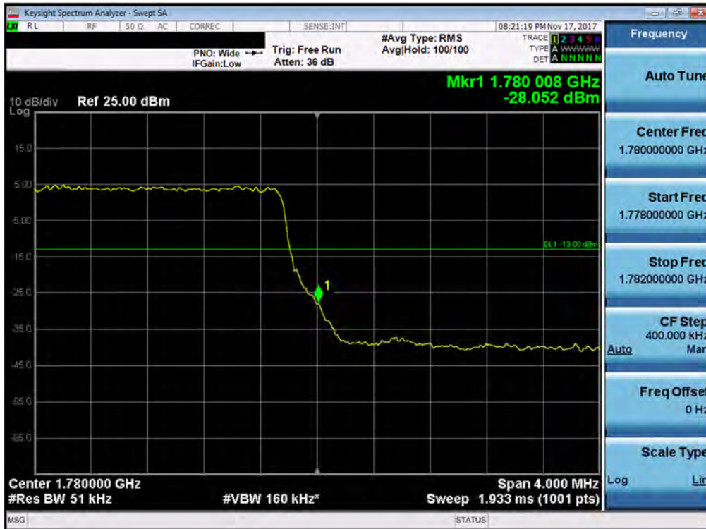
Plot 7-281. Upper Band Edge Plot (Band 66 - 5.0MHz QPSK - Full RB Configuration)
