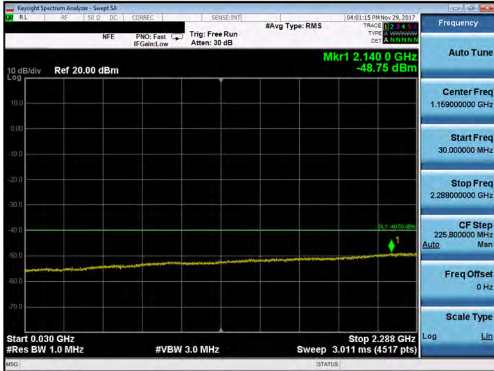
Plot 7-199. Conducted Spurious Plot (Band 30 - 5.0MHz QPSK - RB Size 1, RB Offset 0 - High Channel- Ant B)
