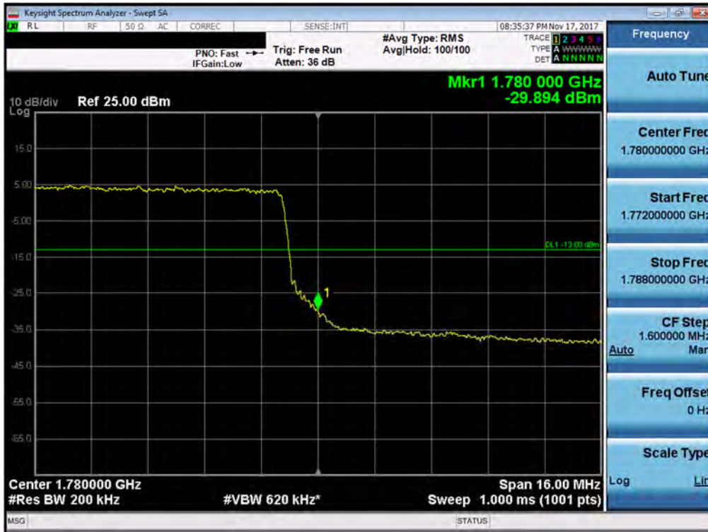
Plot 7-299. Upper Band Edge Plot (Band 66 - 20.0MHz QPSK - Full RB Configuration)
