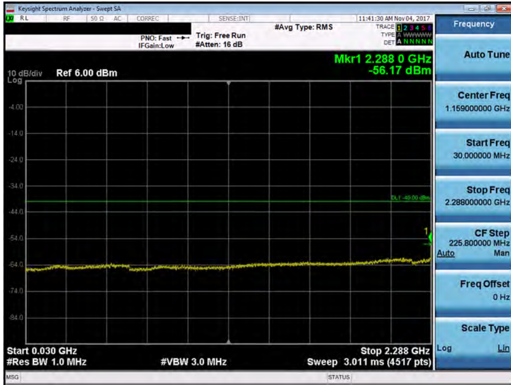
Plot 7-184. Conducted Spurious Plot (Band 30- 5.0MHz QPSK- RB Size 1, RB Offset 0- Low Channel- Ant A)
