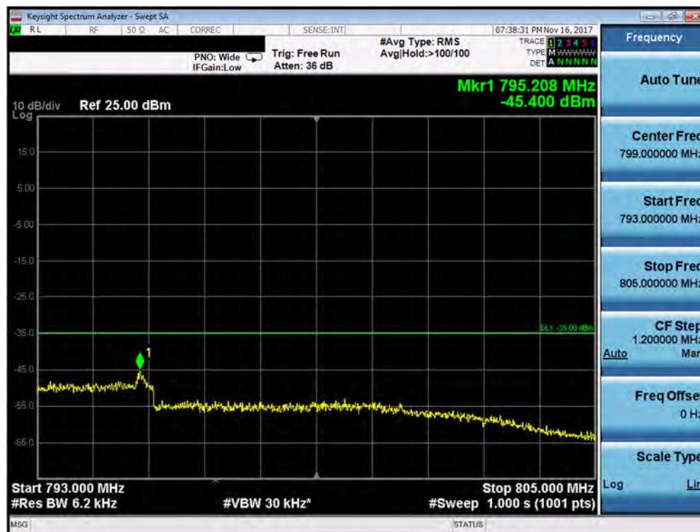
Plot 7-254. Upper Emission Mask Band Edge Plot (Band 13 - 10.0MHz QPSK - Full RB Configuration)
