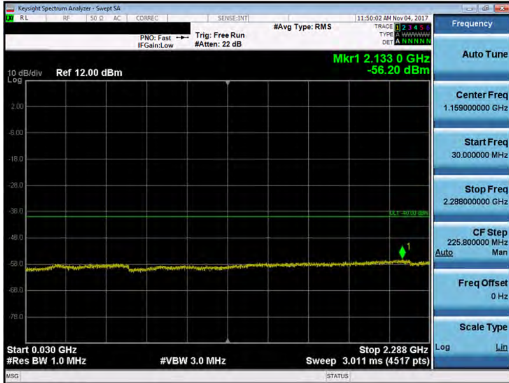
Plot 7-192. Conducted Spurious Plot (Band 30 - 5.0MHz QPSK - RB Size 1, RB Offset 0 - High Channel- Ant A)
