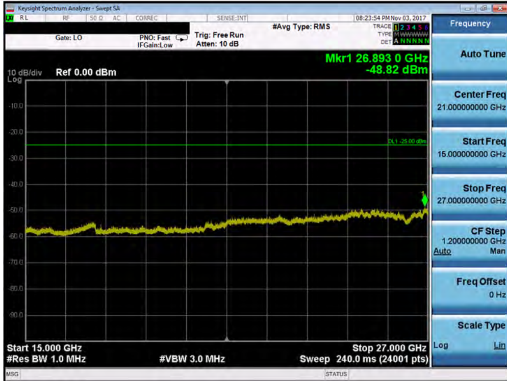
Plot 7-222. Conducted Spurious Plot (Band 38/41- 5.0MHz QPSK- RB Size 1, RB Offset 0- Low Channel)
