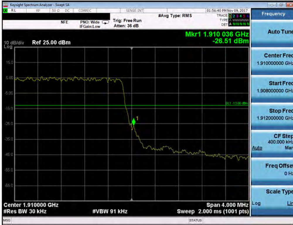
Plot 7-309. Upper Band Edge Plot (Band 2 - 3.0MHz QPSK - Full RB Configuration)
