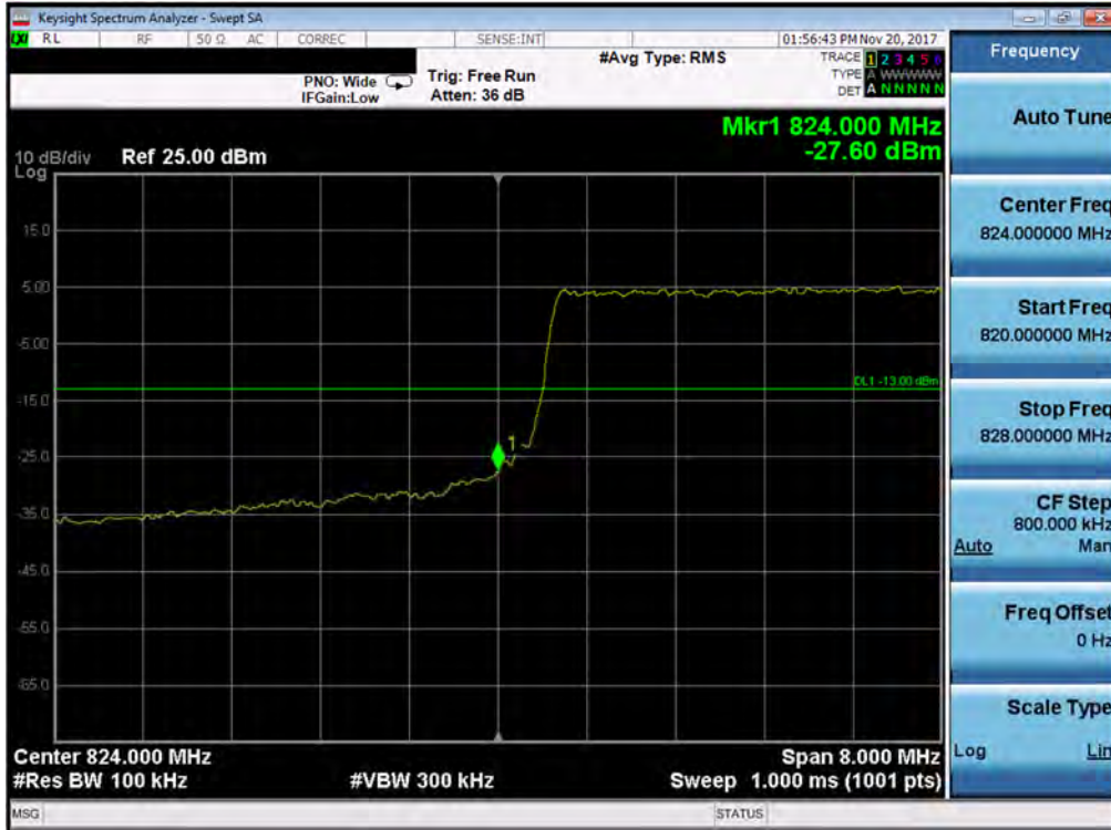
Plot 7-261. Lower Band Edge Plot (Band 5/26 - 10.0MHz QPSK - Full RB Configuration)
