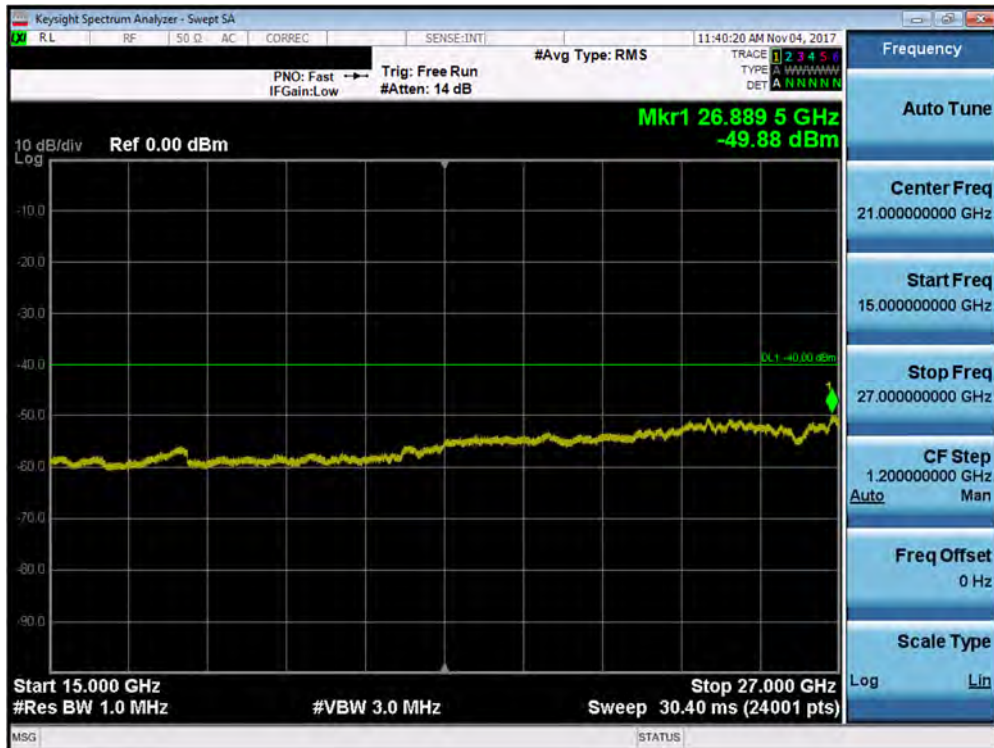
Plot 7-189. Conducted Spurious Plot (Band 30 - 5.0MHz QPSK - RB Size 1, RB Offset 0 - Mid Channel- Ant A)
