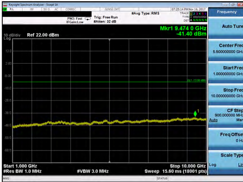
Plot 7-156. Conducted Spurious Plot (Band 13 - 5.0MHz QPSK - RB Size 1, RB Offset 0 - High Channel)
