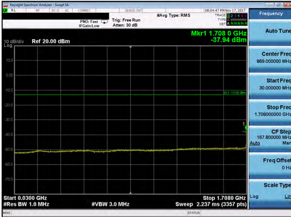
Plot 7-166. Conducted Spurious Plot (Band 4/66 - 1.4MHz QPSK - RB Size 1, RB Offset 0 - Low Channel)
