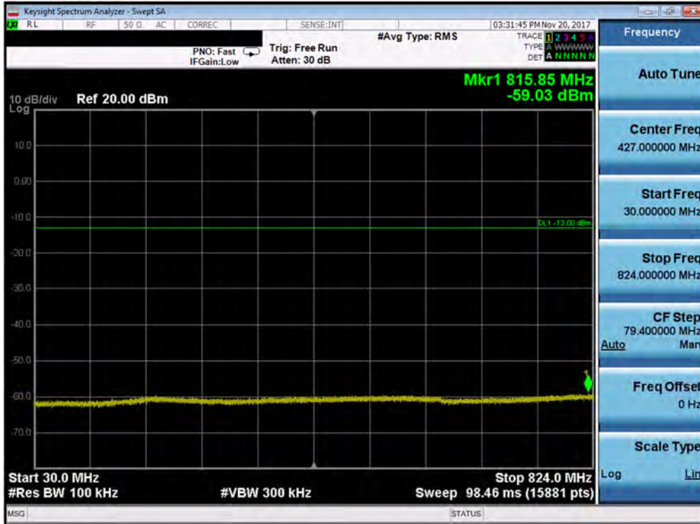
Plot 7-163. Conducted Spurious Plot (Band 5/26 - 3.0MHz QPSK - RB Size 1, RB Offset 0 - High Channel)
