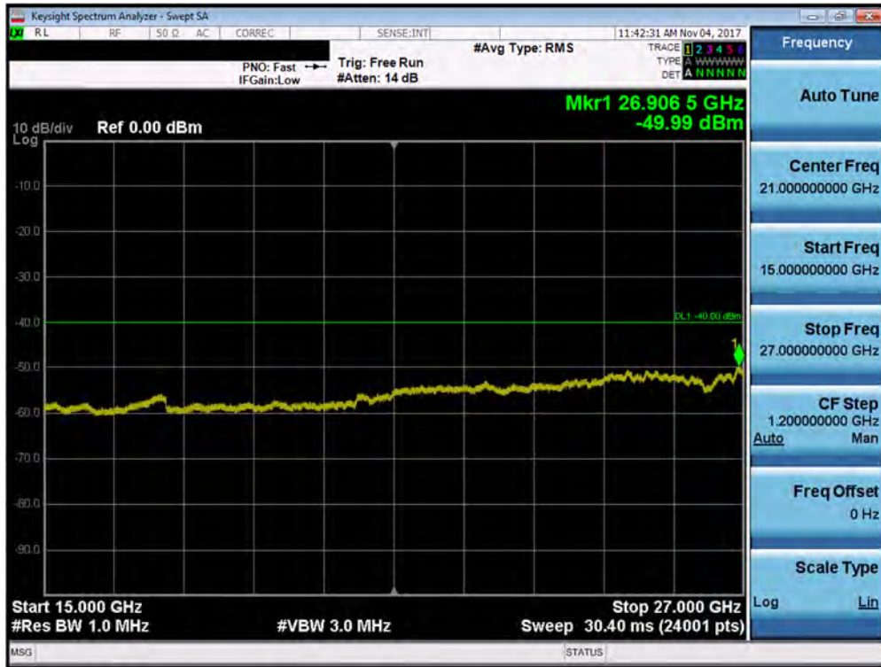
Plot 7-186. Conducted Spurious Plot (Band 30- 5.0MHz QPSK- RB Size 1, RB Offset 0- Low Channel- Ant A)
