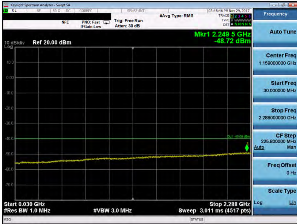
Plot 7-193. Conducted Spurious Plot (Band 30- 5.0MHz QPSK- RB Size 1, RB Offset 0- Low Channel- Ant B)
