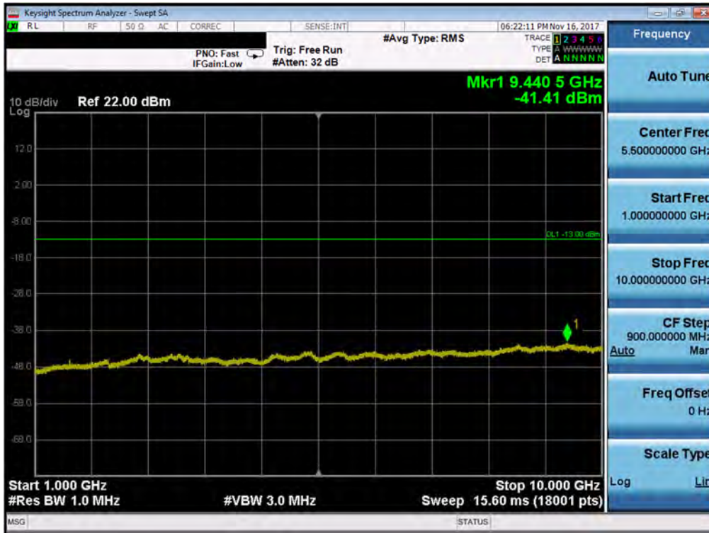
Plot 7-150. Conducted Spurious Plot (Band 13 - 5.0MHz QPSK - RB Size 1, RB Offset 0 - Low Channel)
