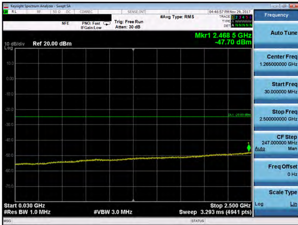
Plot 7-214. Conducted Spurious Plot (Band 7- 5.0MHz QPSK- RB Size 1, RB Offset 0- Mid Channel- Ant B)
