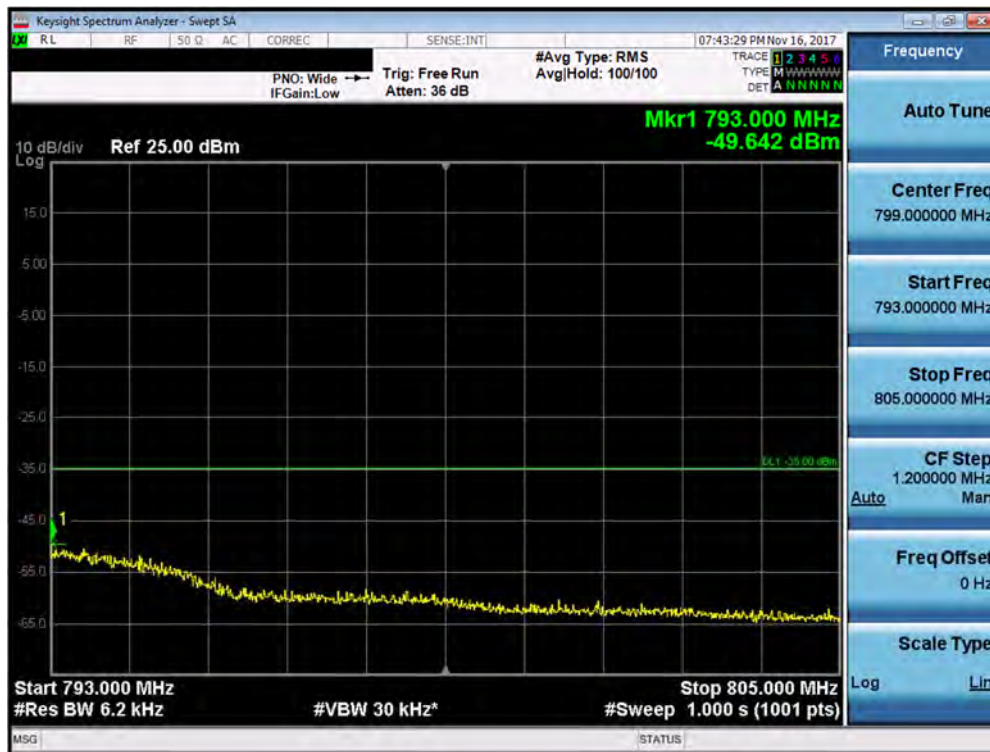
Plot 7-250. Upper Emission Mask Band Edge Plot (Band 13 - 5.0MHz QPSK - Full RB Configuration)
