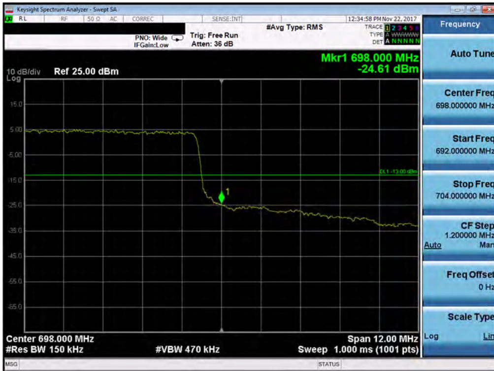
Plot 7-234. Upper Band Edge Plot (Band 71 - 15.0MHz QPSK - Full RB Configuration)
