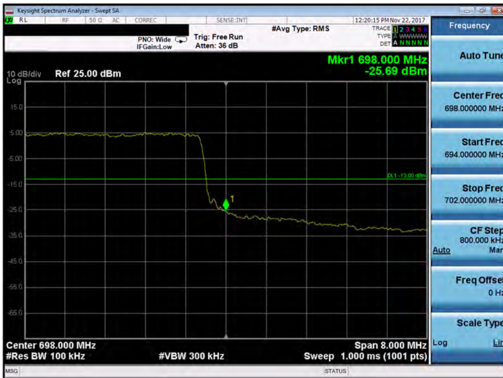
Plot 7-232. Upper Band Edge Plot (Band 71 - 10.0MHz QPSK - Full RB Configuration)
