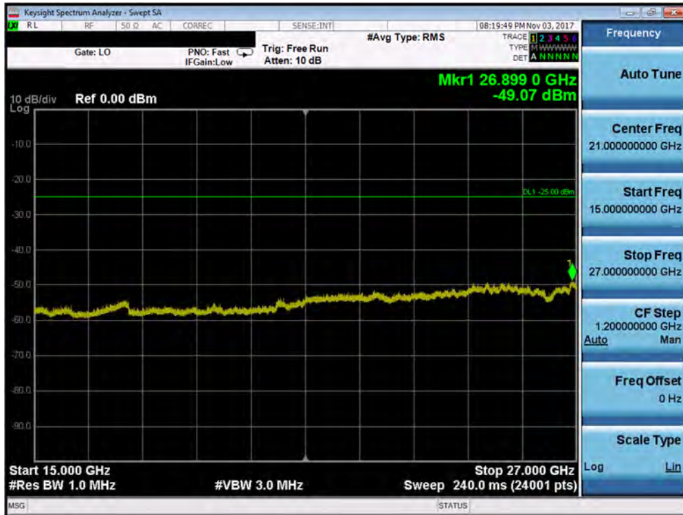
Plot 7-225. Conducted Spurious Plot (Band 38/41- 5.0MHz QPSK- RB Size 1, RB Offset 0- Mid Channel)
