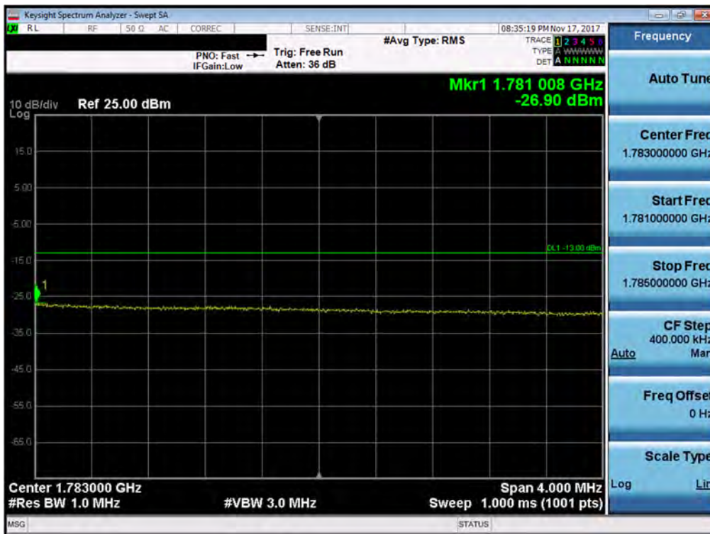
Plot 7-300. Upper Extended Band Edge Plot (Band 66 - 20.0MHz QPSK - Full RB Configuration)
