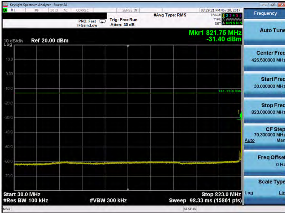
Plot 7-157. Conducted Spurious Plot (Band 5/26 - 3.0MHz QPSK - RB Size 1, RB Offset 0 - Low Channel)
