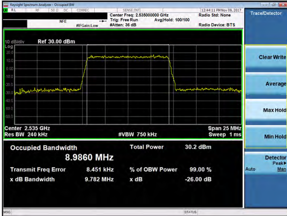
Plot 7-98. Occupied Bandwidth Plot (Band 7 - 10.0MHz 16-QAM - Full RB Configuration- Antenna B)
