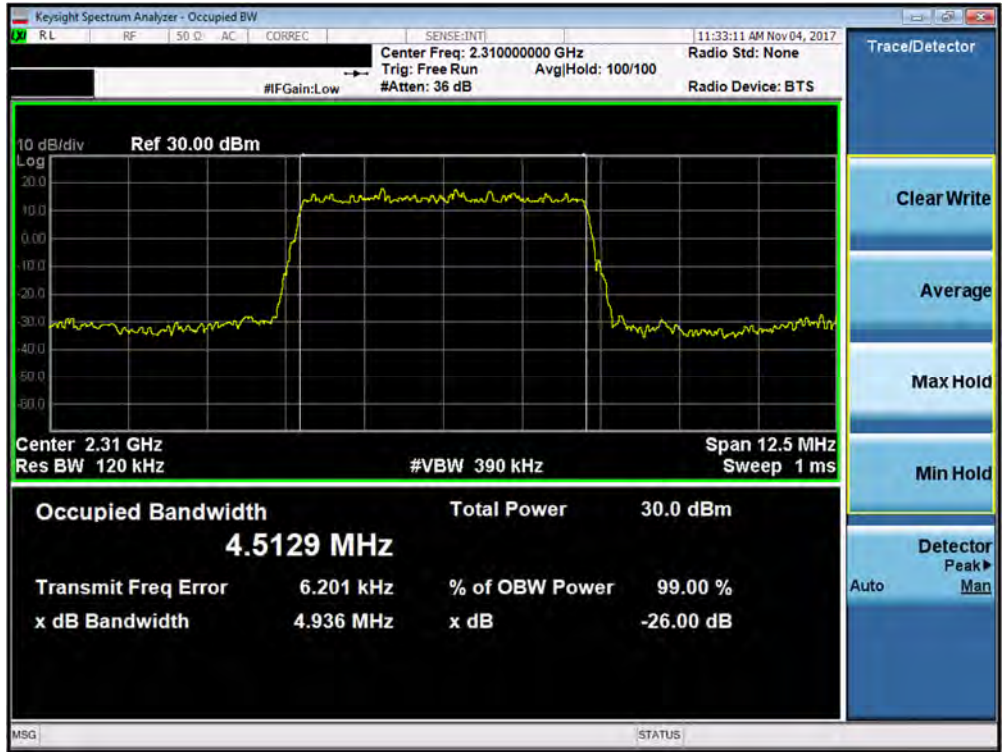
Plot 7-82. Occupied Bandwidth Plot (Band 30 - 5.0MHz QPSK - Full RB Configuration- Antenna B)
