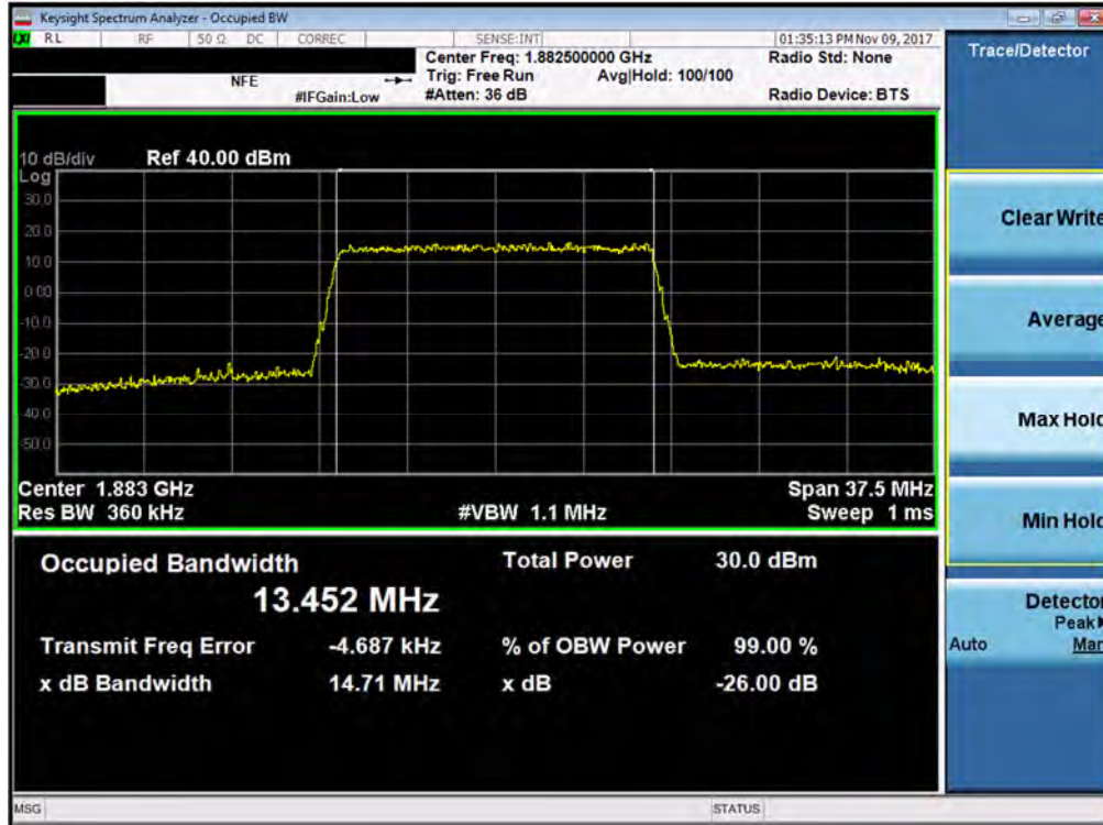
Plot 7-78. Occupied Bandwidth Plot (Band 2/25 - 15.0MHz 64-QAM - Full RB Configuration)
