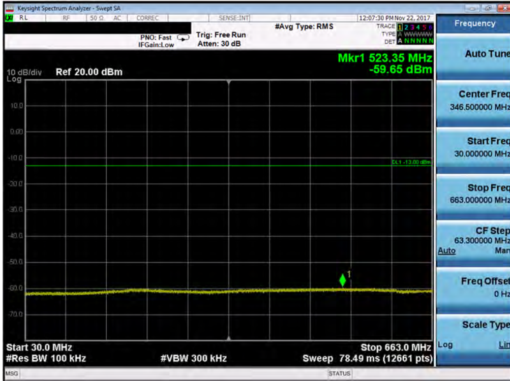
Plot 7-136. Conducted Spurious Plot (Band 71 - 5.0MHz QPSK - RB Size 1, RB Offset 0 - High Channel)
