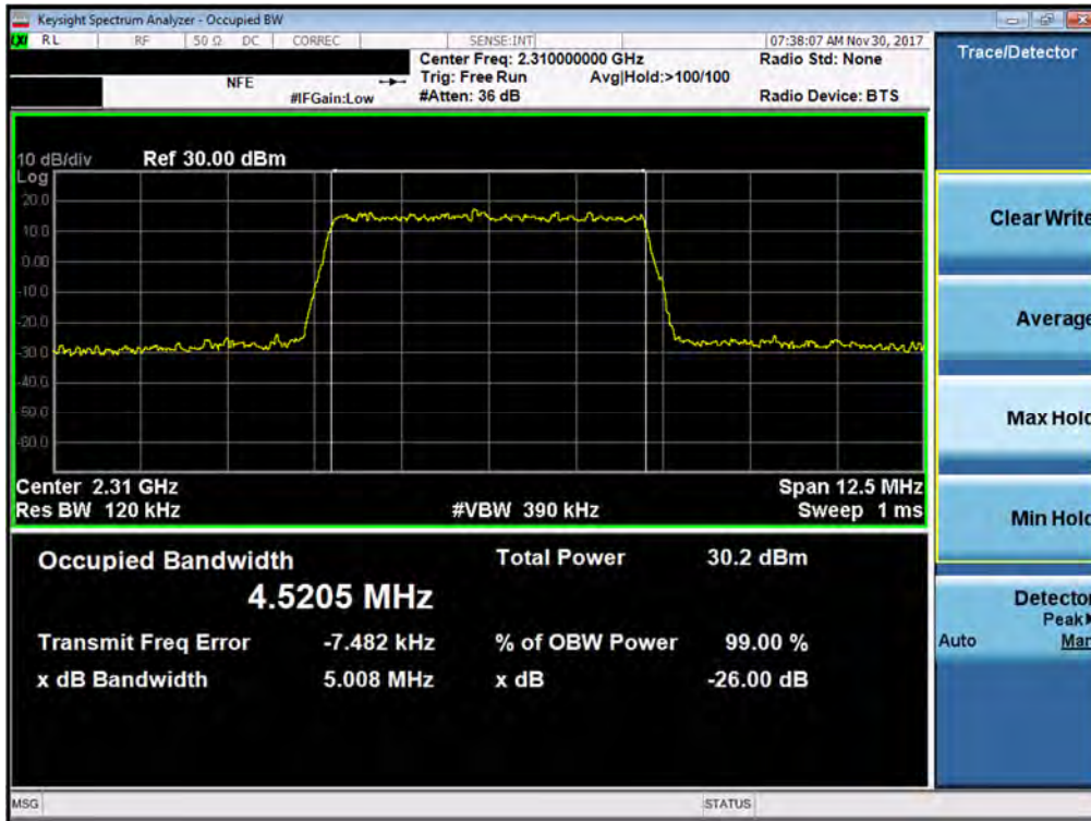
Plot 7-90. Occupied Bandwidth Plot (Band 30 - 5.0MHz 64-QAM - Full RB Configuration- Antenna A)
