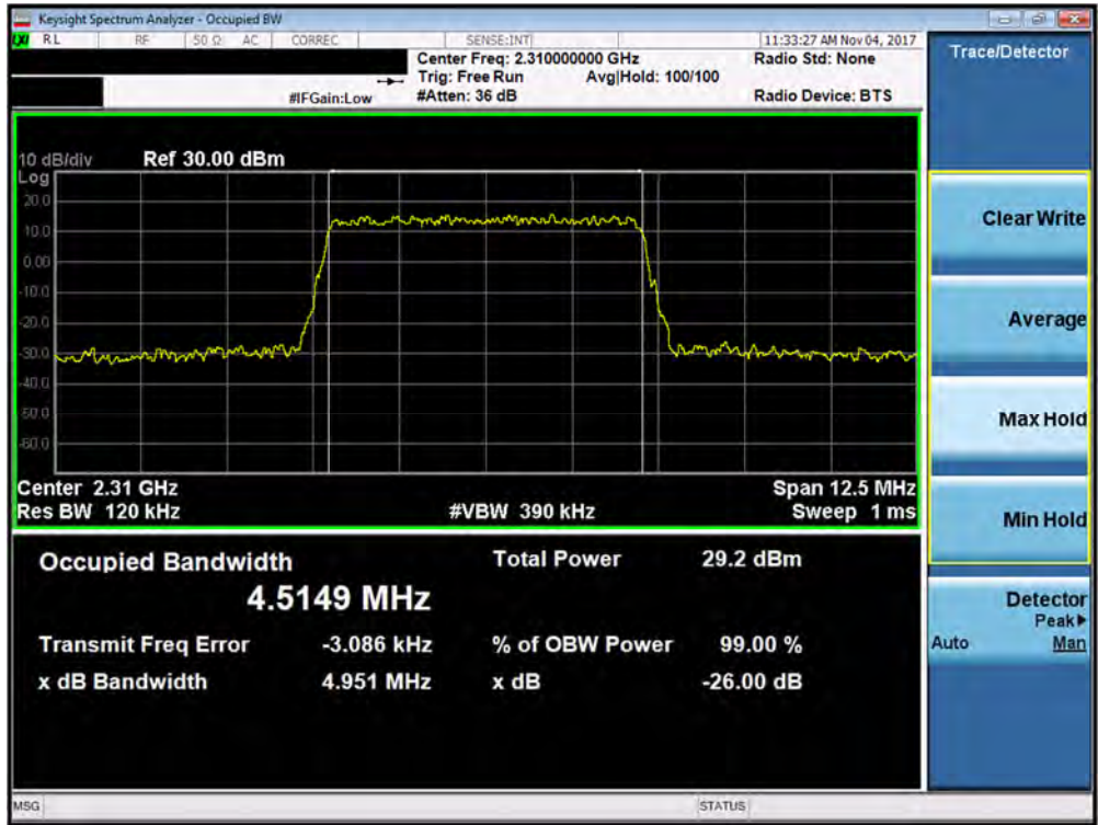
Plot 7-83. Occupied Bandwidth Plot (Band 30 - 5.0MHz 16-QAM - Full RB Configuration- Antenna B)
