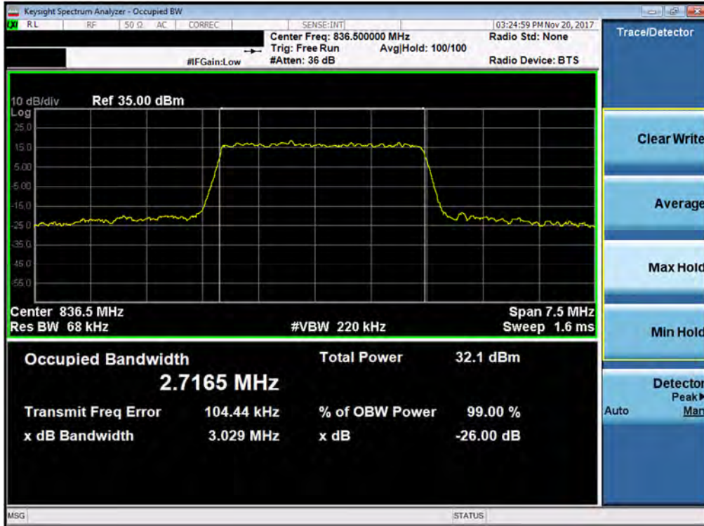
Plot 7-35. Occupied Bandwidth Plot (Band 5/26 - 3.0MHz 16-QAM - Full RB Configuration)
