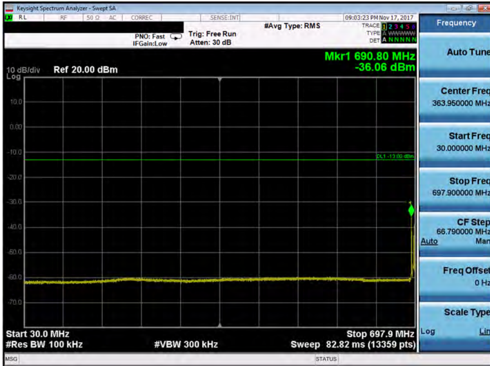
Plot 7-139. Conducted Spurious Plot (Band 12/17 - 10.0MHz QPSK - RB Size 1, RB Offset 0 - Low Channel)
