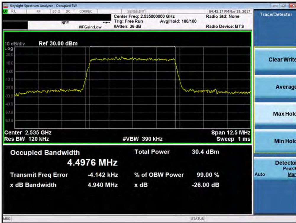
Plot 7-107. Occupied Bandwidth Plot (Band 7 - 5.0MHz 16-QAM - Full RB Configuration- Antenna A)
