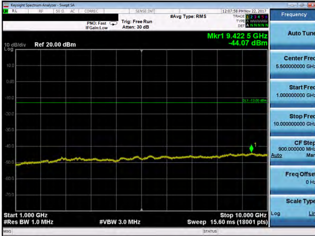
Plot 7-138. Conducted Spurious Plot (Band 71 - 5.0MHz QPSK - RB Size 1, RB Offset 0 - High Channel)
