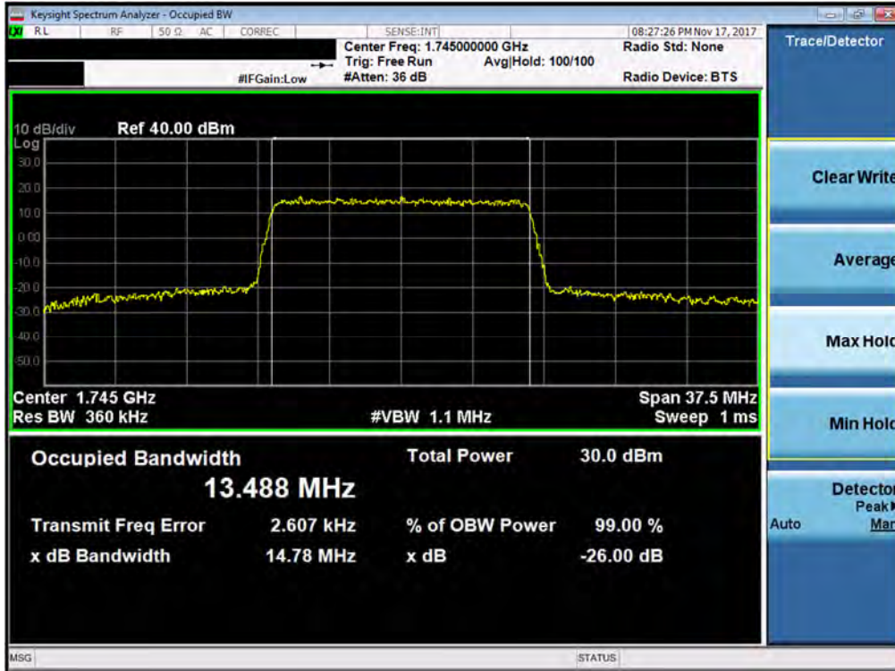
Plot 7-60. Occupied Bandwidth Plot (Band 4/66 - 15.0MHz 64-QAM - Full RB Configuration)
