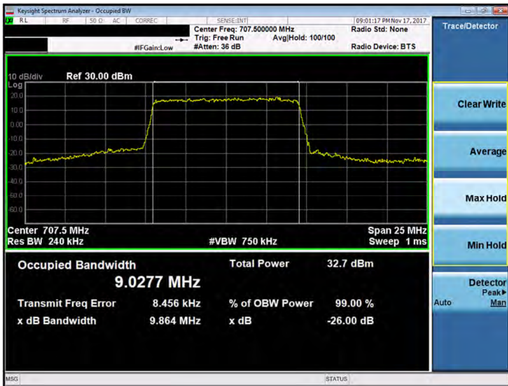
Plot 7-22. Occupied Bandwidth Plot (Band 12/17 - 10.0MHz QPSK - Full RB Configuration)
