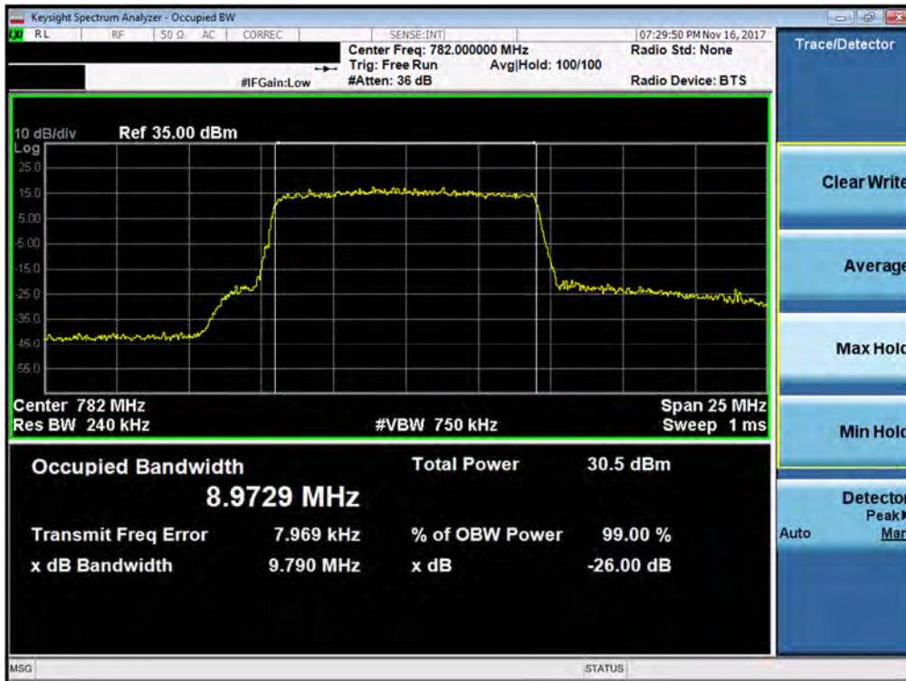
Plot 7-30. Occupied Bandwidth Plot (Band 13 - 10.0MHz 64-QAM - Full RB Configuration)
