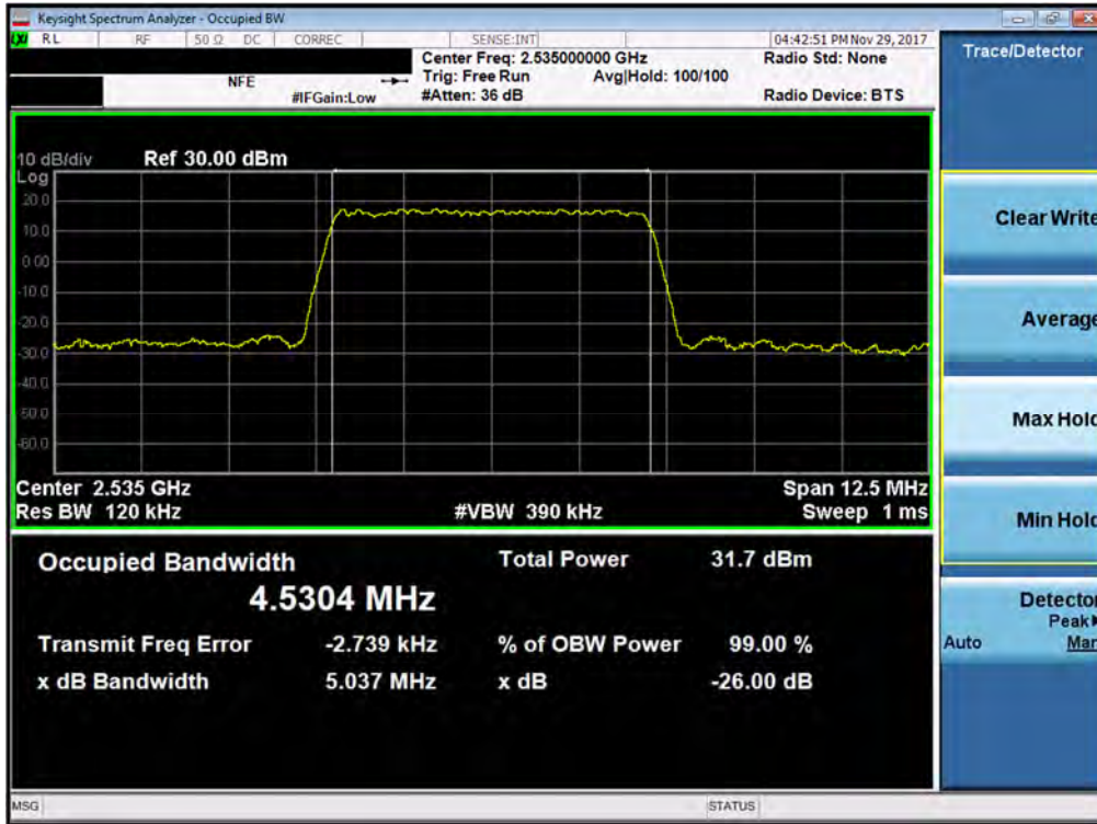
Plot 7-106. Occupied Bandwidth Plot (Band 7 - 5.0MHz QPSK - Full RB Configuration- Antenna A)
