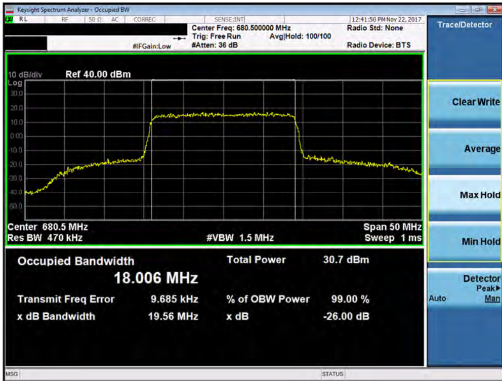
Plot 7-12. Occupied Bandwidth Plot (Band 71 - 20.0MHz 64-QAM - Full RB Configuration)
