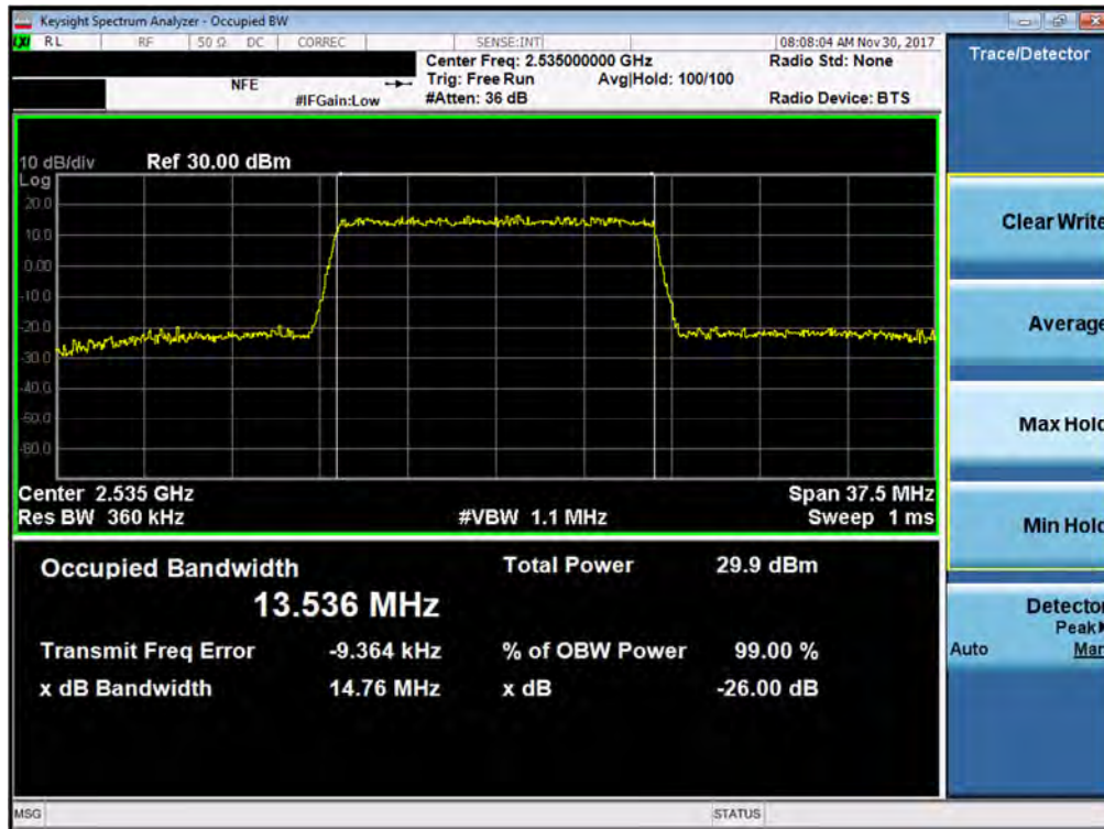
Plot 7-113. Occupied Bandwidth Plot (Band 7 - 15.0MHz 16-QAM - Full RB Configuration- Antenna A)
