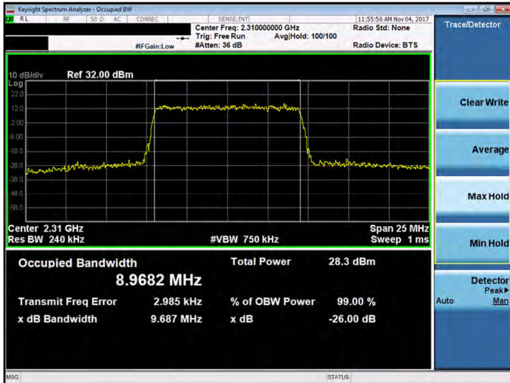
Plot 7-87. Occupied Bandwidth Plot (Band 30 - 10.0MHz 64-QAM - Full RB Configuration- Antenna B)
