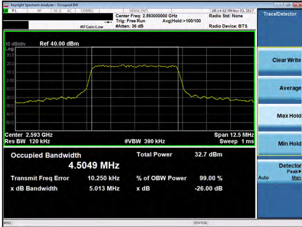
Plot 7-120. Occupied Bandwidth Plot (Band 38/41 - 5.0MHz 64-QAM - Full RB Configuration)
