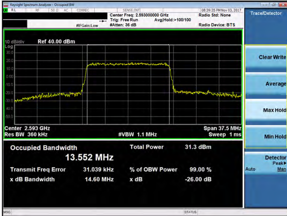
Plot 7-126. Occupied Bandwidth Plot (Band 38/41 - 15.0MHz 64-QAM - Full RB Configuration)
