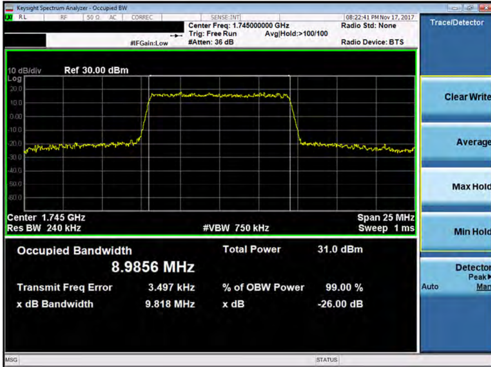
Plot 7-56. Occupied Bandwidth Plot (Band 4/66 - 10.0MHz 16-QAM - Full RB Configuration)
