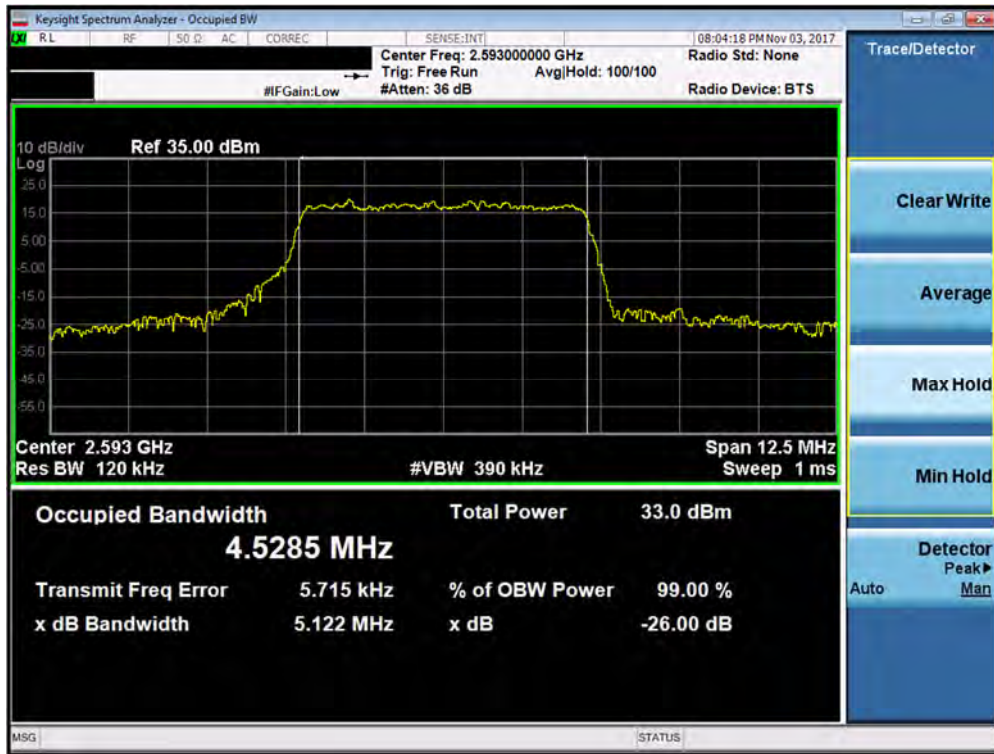
Plot 7-119. Occupied Bandwidth Plot (Band 38/41 - 5.0MHz 16-QAM - Full RB Configuration)
