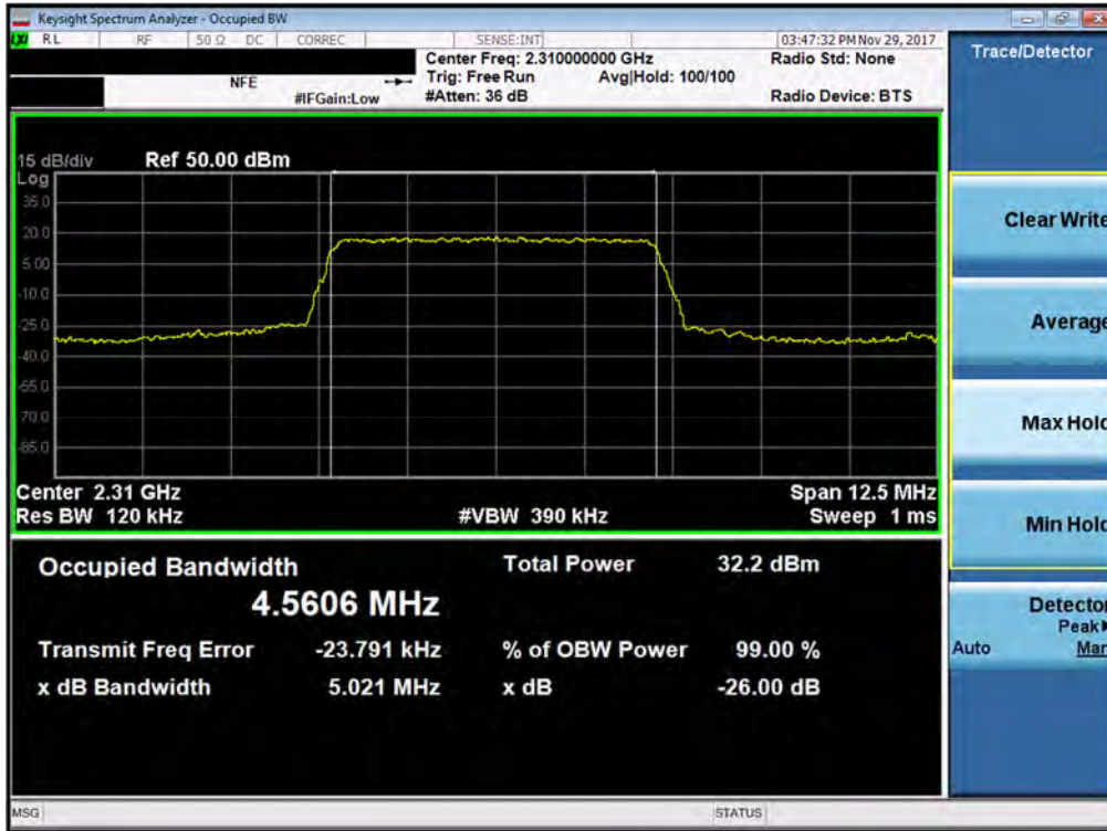
Plot 7-88. Occupied Bandwidth Plot (Band 30 - 5.0MHz QPSK - Full RB Configuration- Antenna A)
