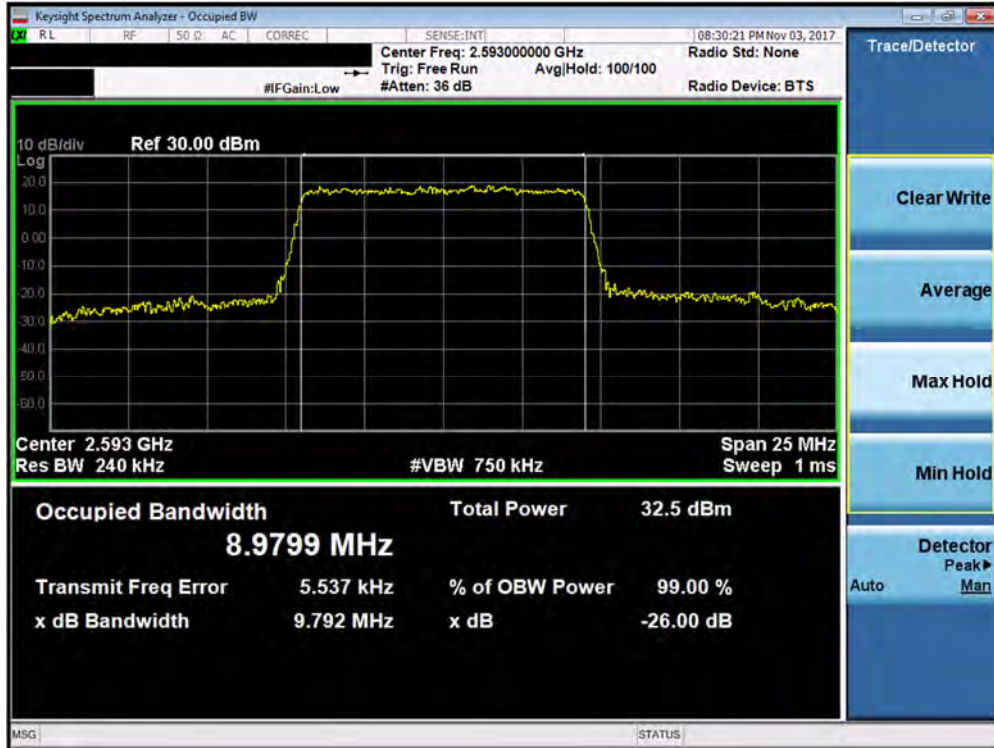
Plot 7-122. Occupied Bandwidth Plot (Band 38/41 - 10.0MHz 16-QAM - Full RB Configuration)
