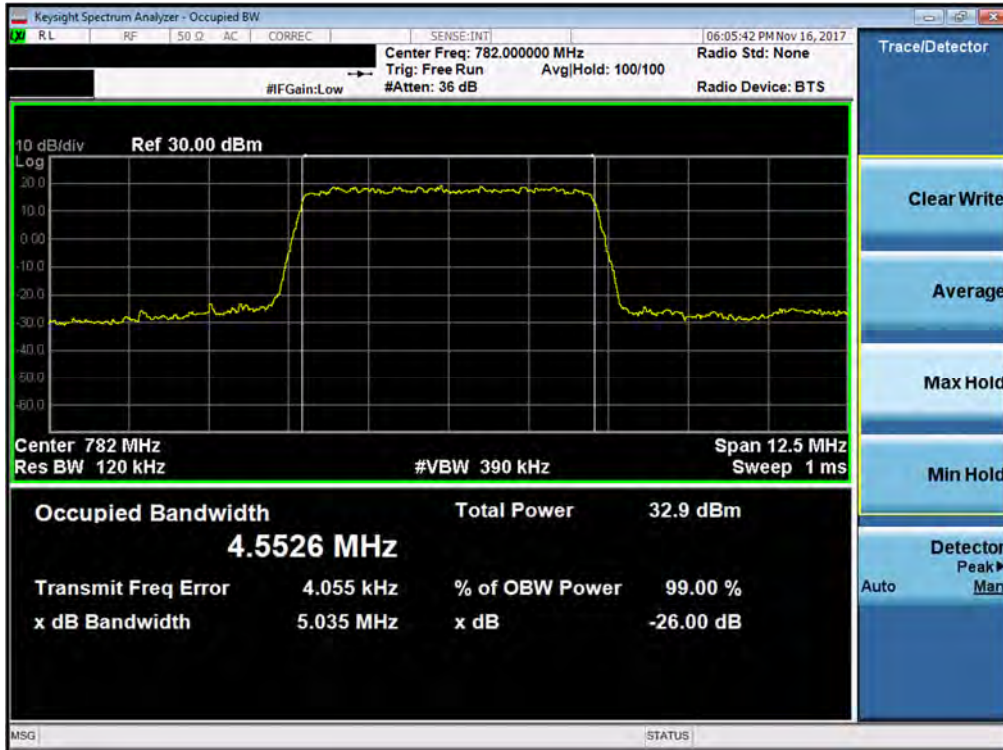
Plot 7-25. Occupied Bandwidth Plot (Band 13 - 5.0MHz QPSK - Full RB Configuration)
