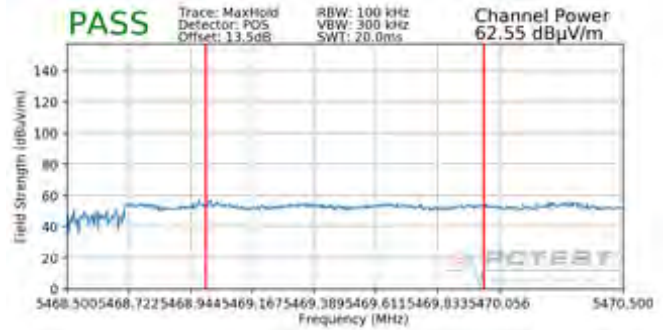
Plot 7-218. Radiated Lower Band Edge Plot (Peak – UNII Band 2C)
