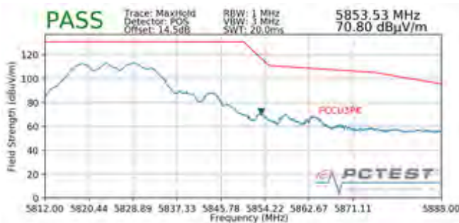
Plot 7-282. Radiated Upper Band Edge Plot (Peak – UNII Band 3)
