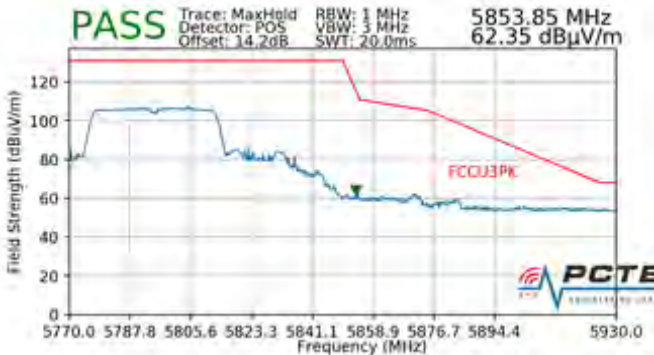
Plot 7-237. Radiated Upper Band Edge Plot (Peak – UNII Band 3)
