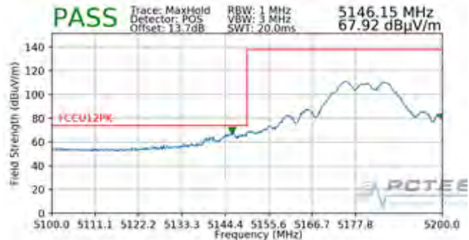
Plot 7-277. Radiated Lower Band Edge Plot (Peak – UNII Band 1)
