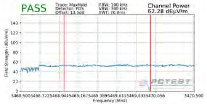
Plot 7-200. Radiated Lower Band Edge Plot (Peak – UNII Band 2C)
