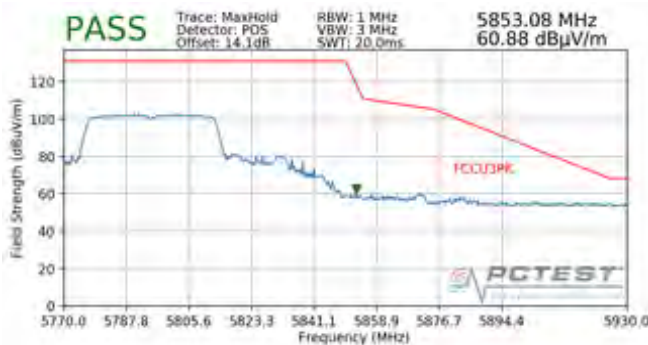
Plot 7-210. Radiated Upper Band Edge Plot (Peak – UNII Band 3)
