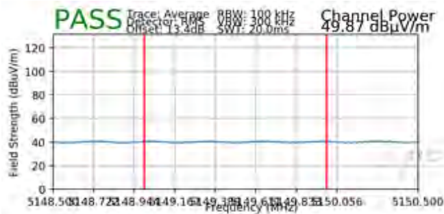
Plot 7-240. Radiated Lower Band Edge Plot (Average – UNII Band 1)
