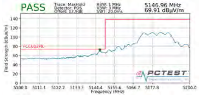
Plot 7-284. Radiated Band Edge Plot (Peak – WCP)
