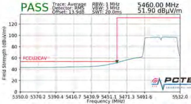
Plot 7-235. Radiated Lower Band Edge Plot (Average – UNII Band 2C)
