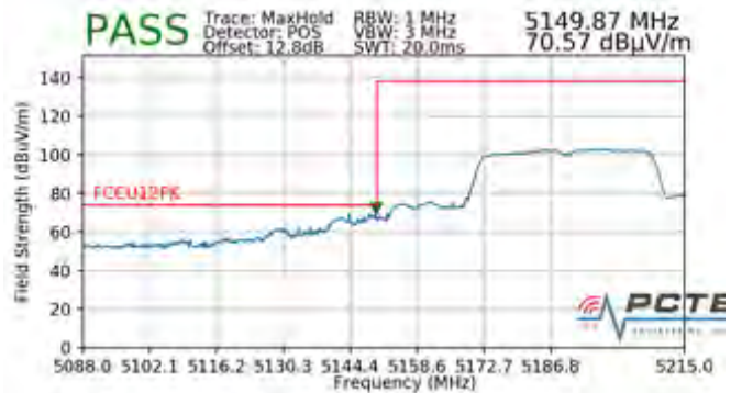
Plot 7-232. Radiated Lower Band Edge Plot (Peak – UNII Band 1)
