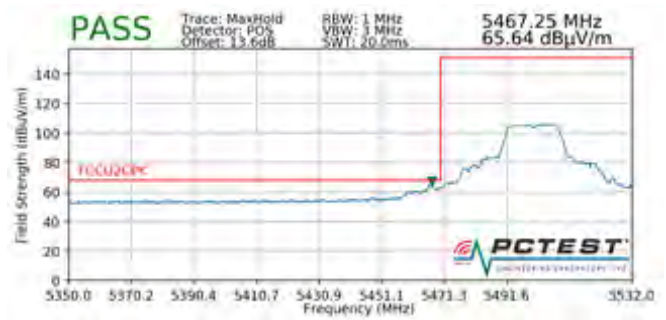
Plot 7-212. Radiated Band Edge Plot (Peak – WCP)
