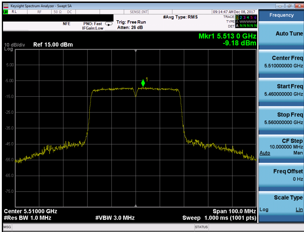
Plot 7-101. Power Spectral Density Plot (40MHz BW 802.11n (UNII Band 2C) – Ch. 102)
