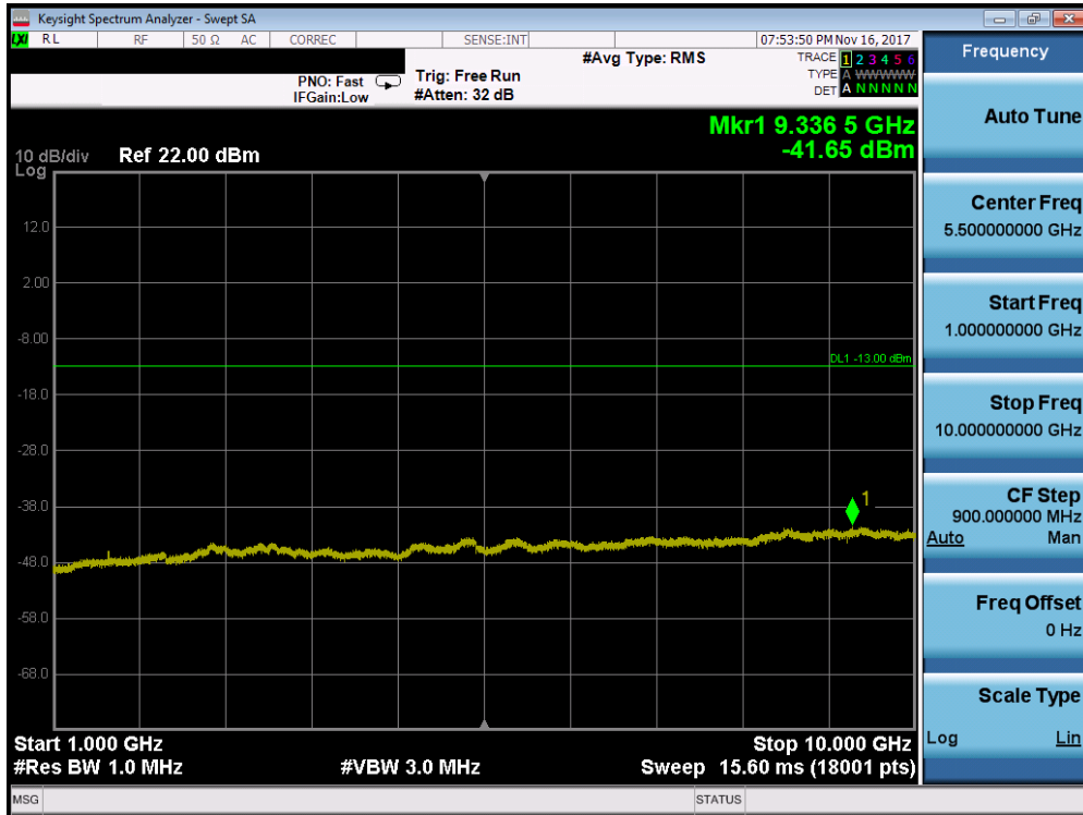
Plot 7-30. Conducted Spurious Plot (LTE B14 – 5.0MHz QPSK – RB Size 1, RB Offset 0 – Low Channel)
