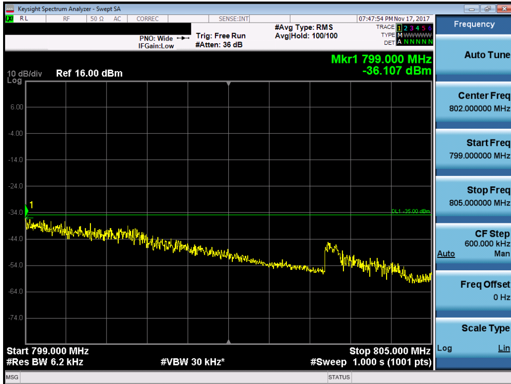
Plot 7-50. Upper Emission Mask Band Edge Plot (LTE B14 - 10MHz QPSK – RB Size 50)
