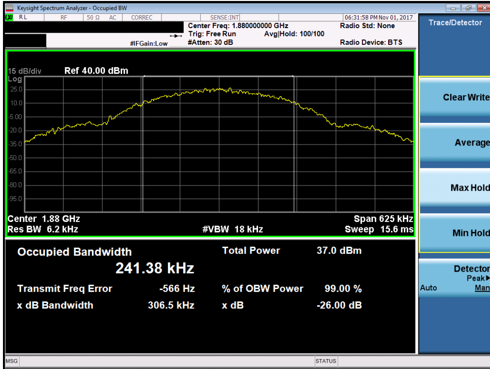
Plot 7-3. Occupied Bandwidth Plot (PCS GPRS Mode)
