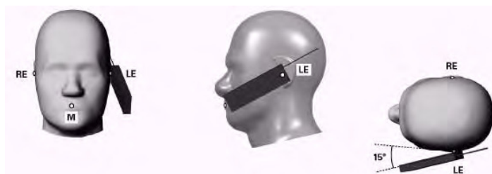
Figure 5-2 Front, Side and Top View of Ear/15° Tilt Position
