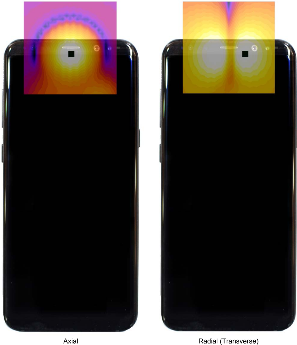
Figure 13-3 T-Coil Scan Overlay Magnetic Field Distributions
