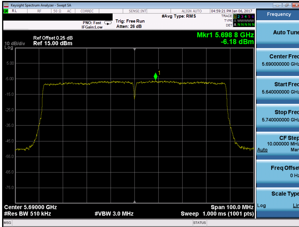
Plot 7-146. Power Spectral Density Plot (80MHz BW 802.11ac (UNII Band 2C) – Ch. 138)
