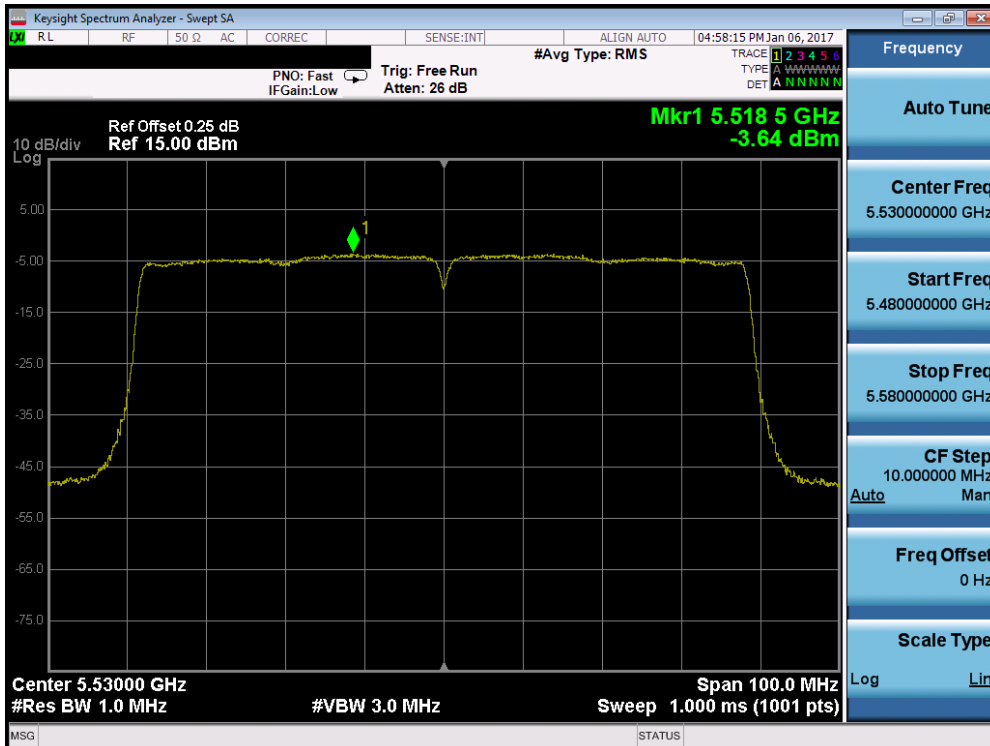
Plot 7-145. Power Spectral Density Plot (80MHz BW 802.11ac (UNII Band 2C) – Ch. 106)
