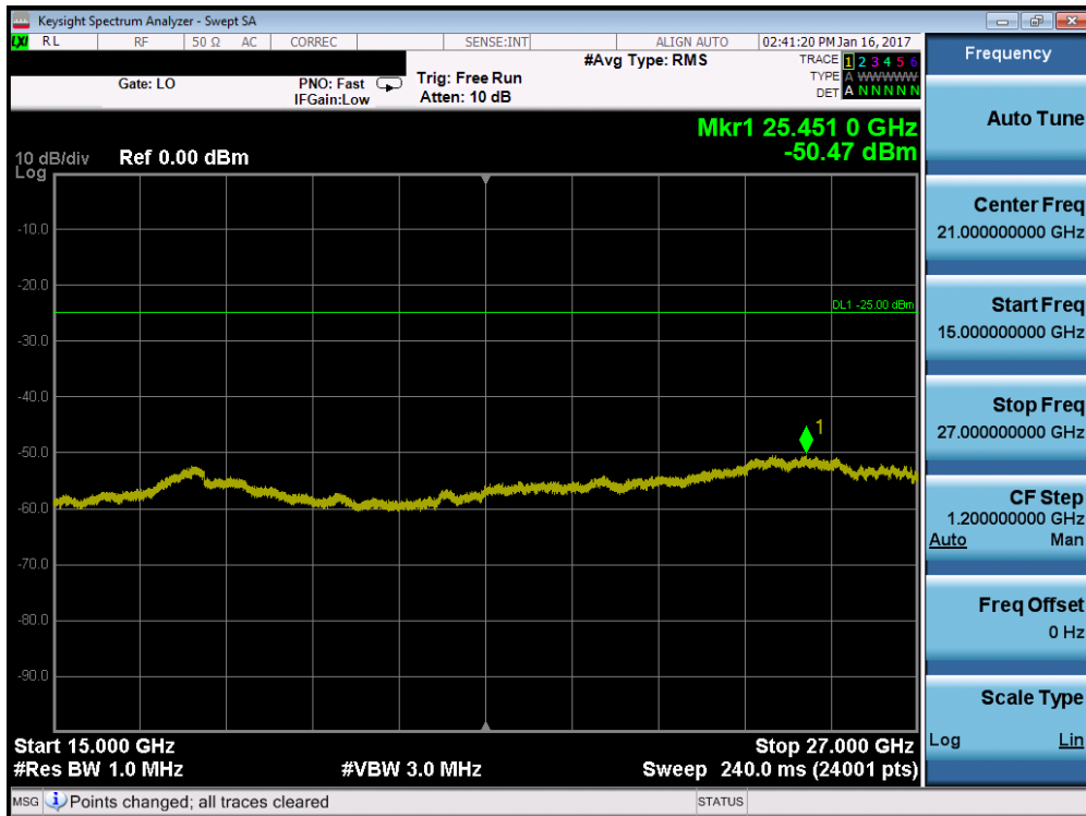
Plot 7-102. Conducted Spurious Plot (Band 41 – 5.0MHz QPSK – RB Size 1, RB Offset 0 – High Channel)
