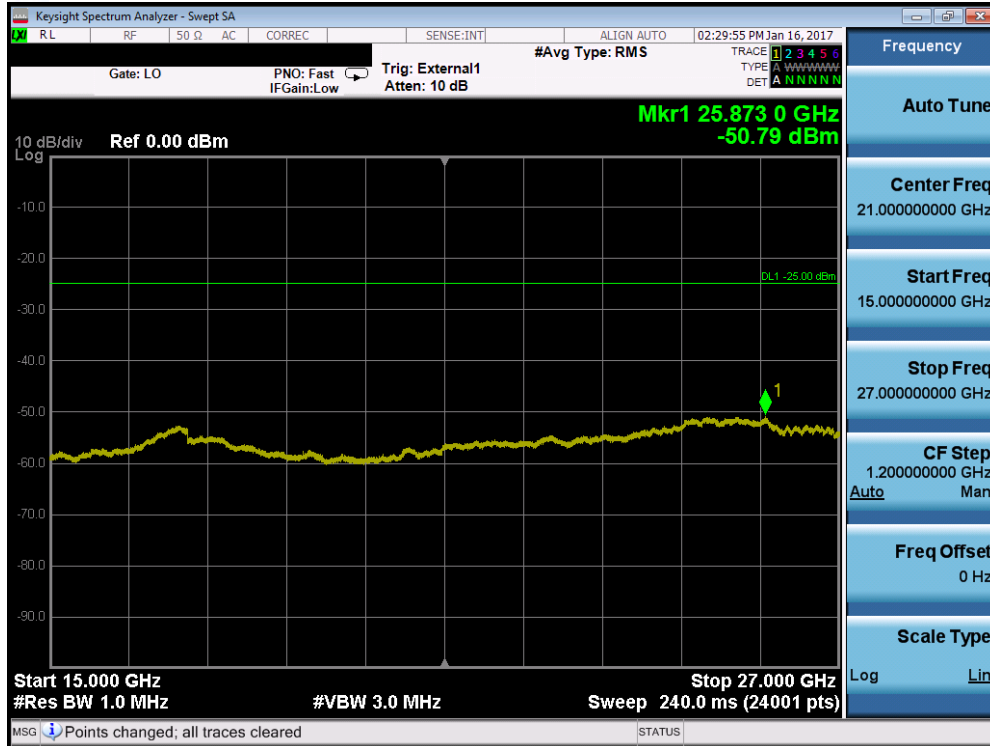
Plot 7-99. Conducted Spurious Plot (Band 41 – 5.0MHz QPSK – RB Size 1, RB Offset 0 – Mid Channel)
