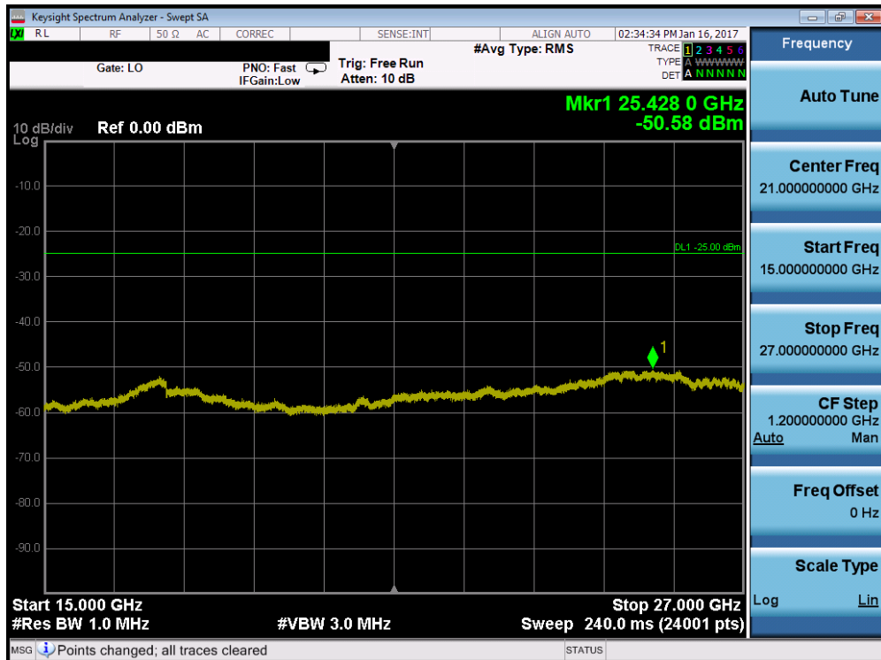
Plot 7-96. Conducted Spurious Plot (Band 41 – 5.0MHz QPSK – RB Size 1, RB Offset 0 – Low Channel)
