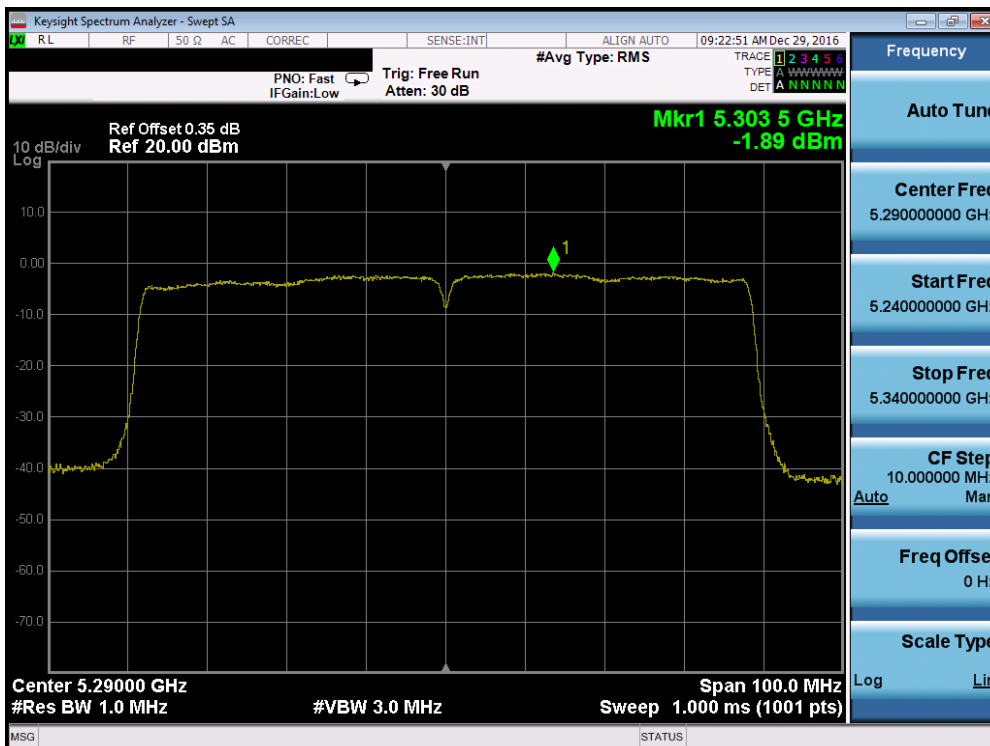
Plot 7-135. Power Spectral Density Plot (80MHz BW 802.11ac (UNII Band 2A) – Ch. 58)
