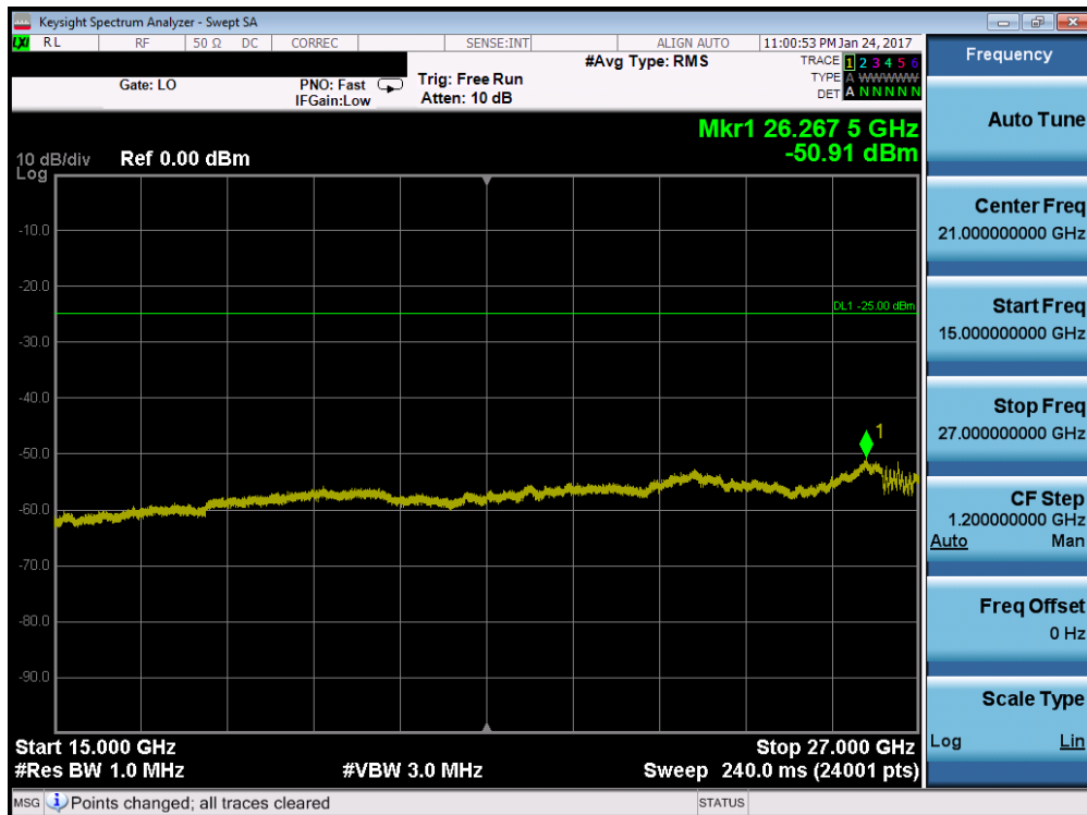
Plot 7-135. Conducted Spurious Plot (Band 41 – 10.0MHz QPSK – RB Size 1, RB Offset 0 – High Channel)
