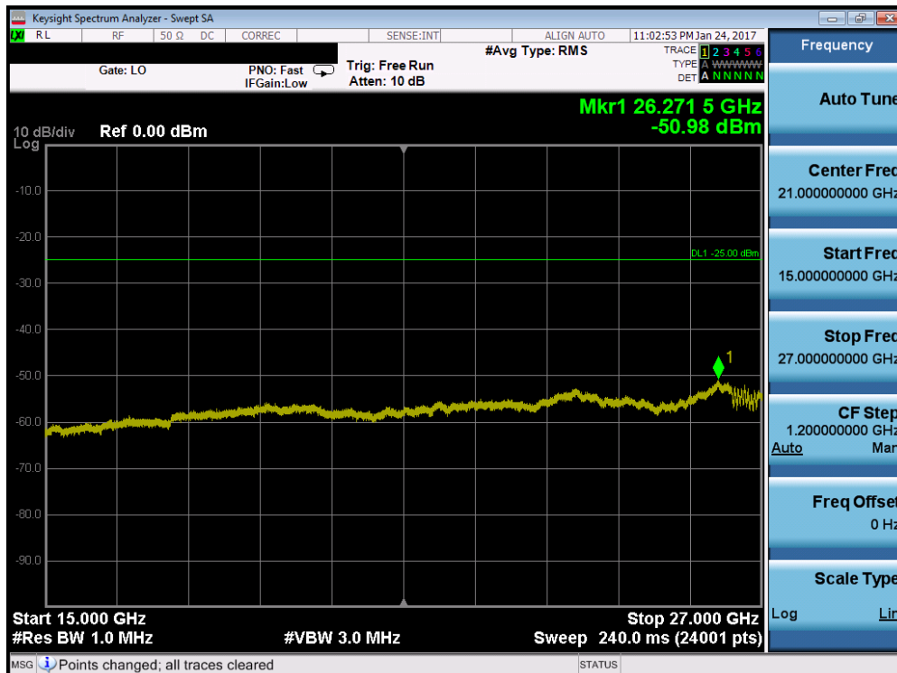
Plot 7-129. Conducted Spurious Plot (Band 41 – 10.0MHz QPSK – RB Size 1, RB Offset 0 – Low Channel)
