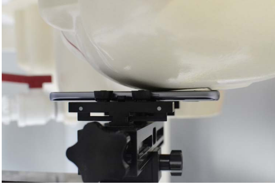
SAR Test Setup Photo 3: Left Cheek
