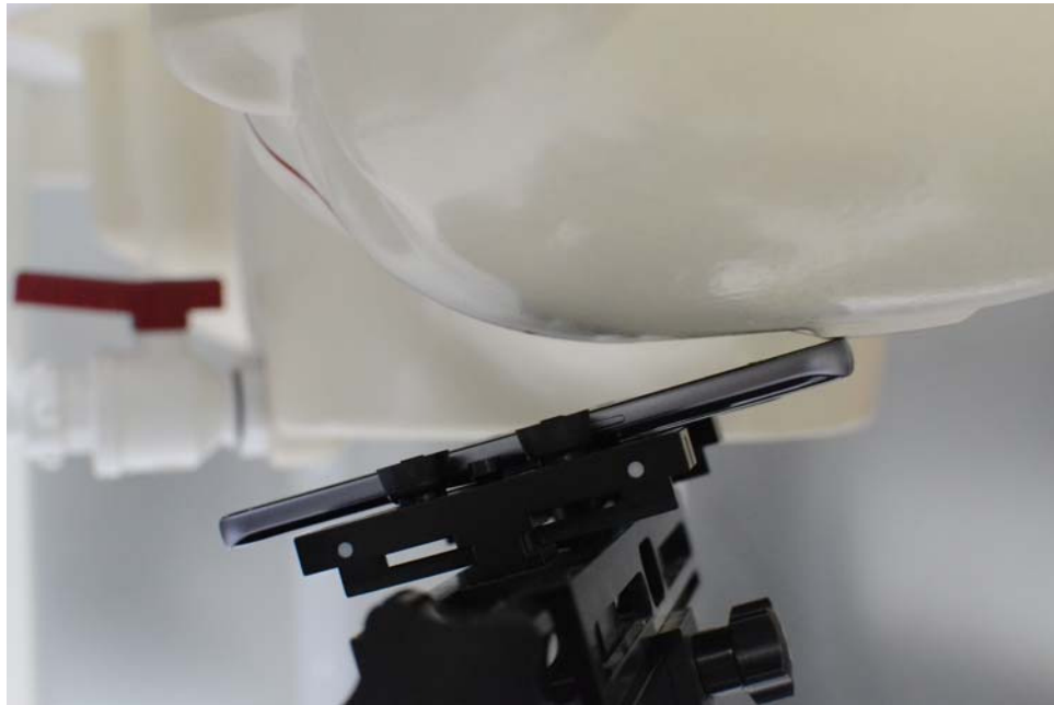
SAR Test Setup Photo 4: Left Tilt
