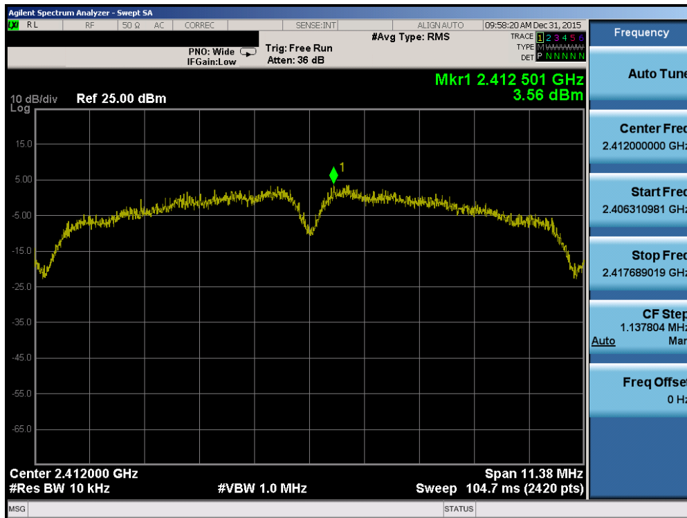
Plot 7-19. Power Spectral Density Plot (802.11b – Ch. 1)
