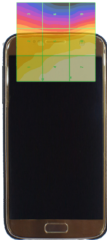
Figure 15-4 E-Field WD Scan overlay
