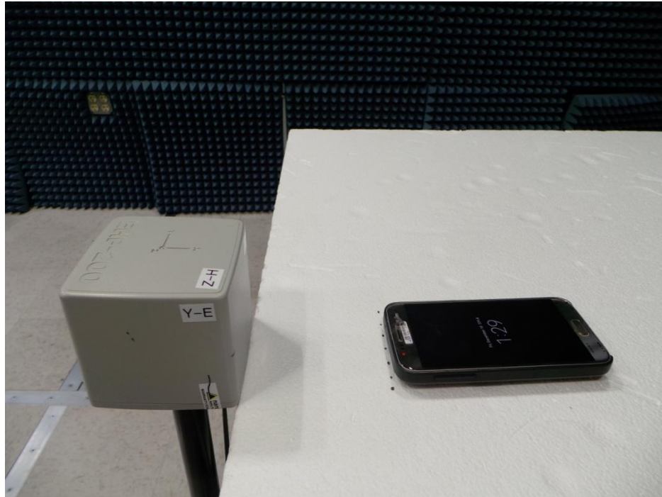
Figure 1. E-Field Measurement (Position A)
