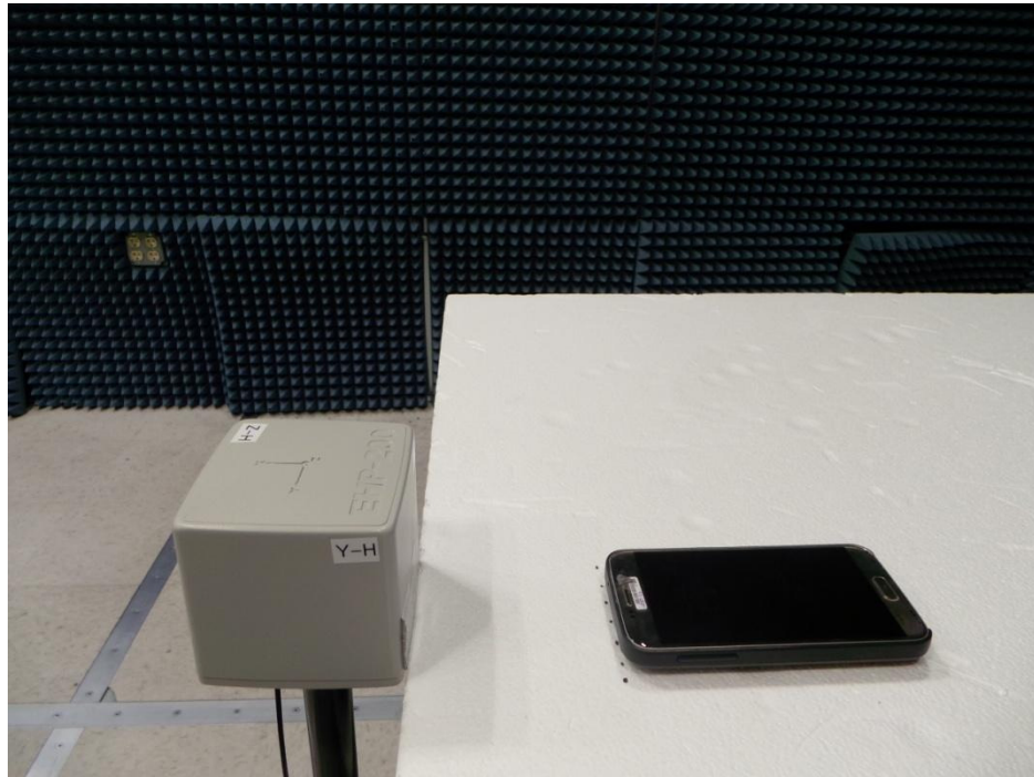
Figure 7. H-Field Measurement (Position A)
