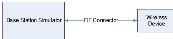
Figure 9-3 Power Measurement Setup
