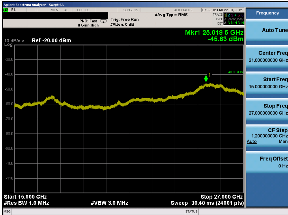
Plot 7-106. Conducted Spurious Plot (Band 30 – 10.0MHz QPSK – RB Size 1, RB Offset 0 – Mid Channel)
