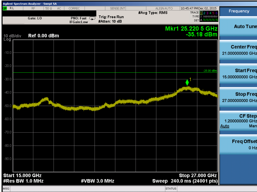
Plot 7-115. Conducted Spurious Plot (Band 41 – 15.0MHz QPSK – RB Size 1, RB Offset 0 – High Channel)
