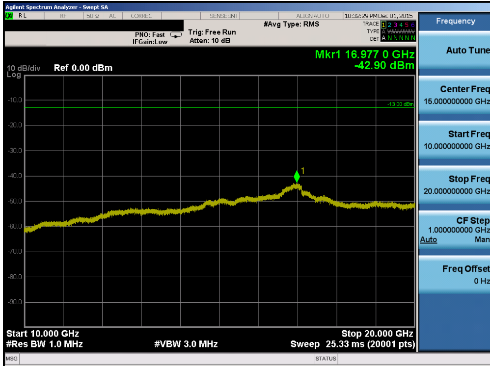
Plot 7-97. Conducted Spurious Plot (Band 2/25 – 1.4MHz QPSK – RB Size 1, RB Offset 0 – Low Channel)
