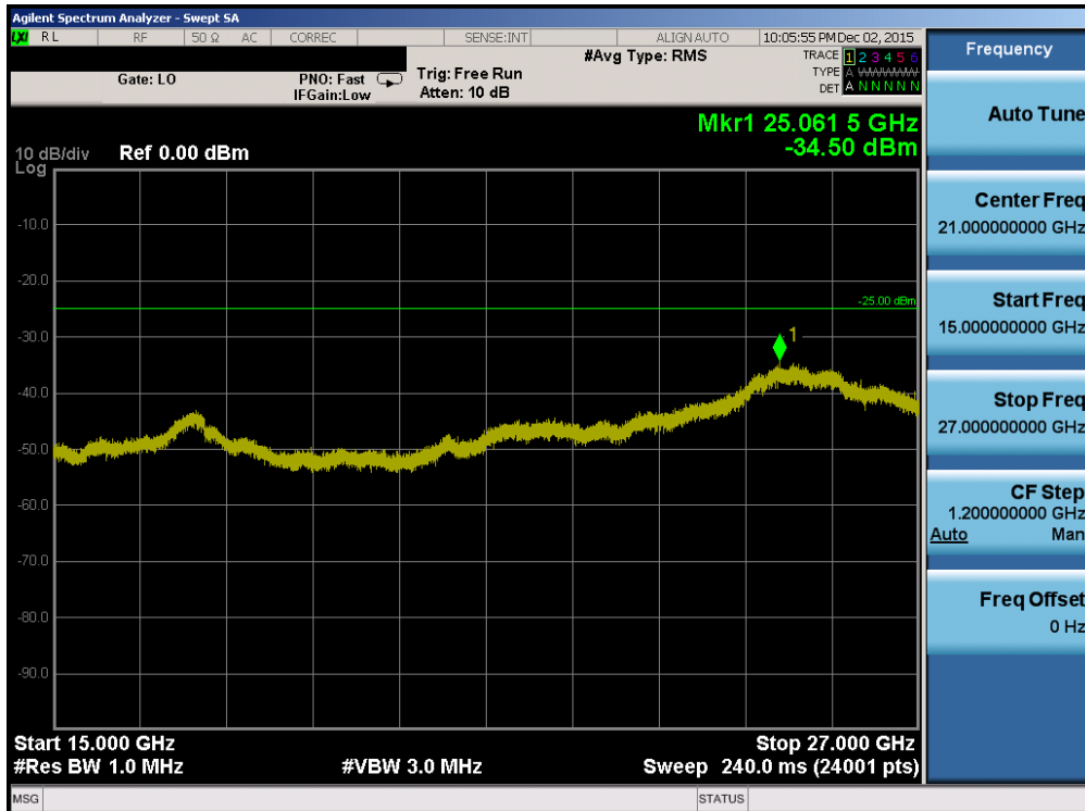
Plot 7-112. Conducted Spurious Plot (Band 41 – 15.0MHz QPSK – RB Size 1, RB Offset 0 – Mid Channel)
