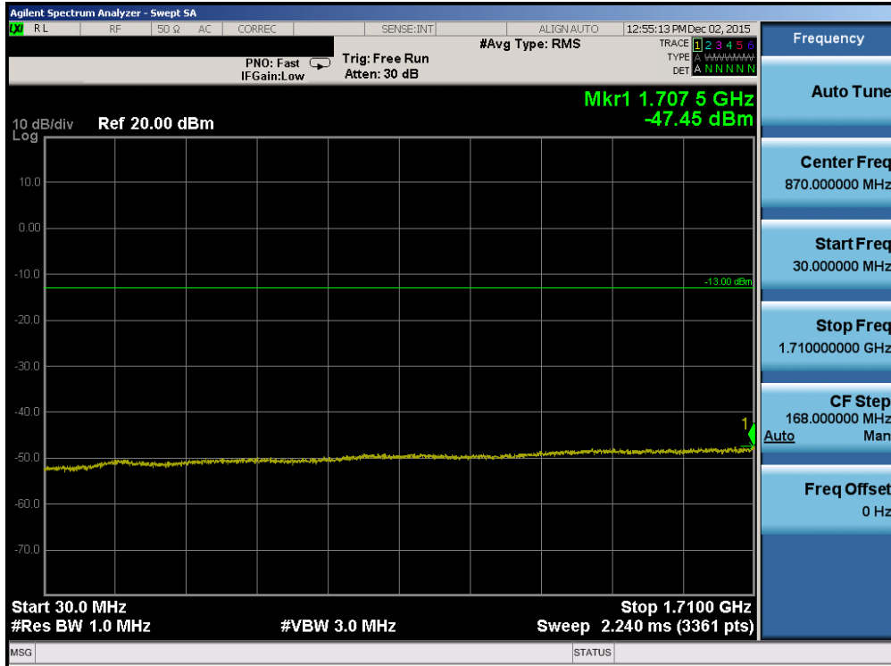
Plot 7-89. Conducted Spurious Plot (Band 4 – 3.0MHz QPSK – RB Size 1, RB Offset 0 – Mid Channel)
