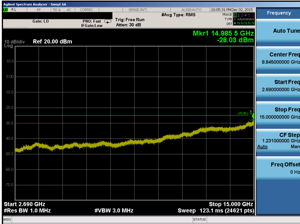
Plot 7-111. Conducted Spurious Plot (Band 41 – 15.0MHz QPSK – RB Size 1, RB Offset 0 – Mid Channel)
