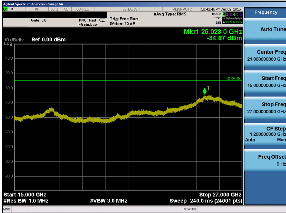
Plot 7-109. Conducted Spurious Plot (Band 41 – 15.0MHz QPSK – RB Size 1, RB Offset 0 – Low Channel)
