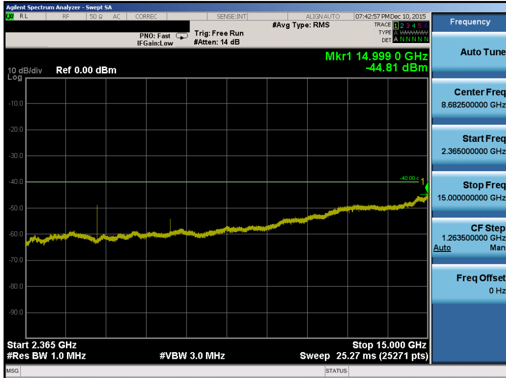
Plot 7-105. Conducted Spurious Plot (Band 30 – 10.0MHz QPSK – RB Size 1, RB Offset 0 – Mid Channel)
