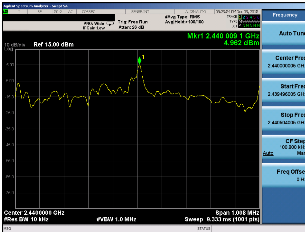
Plot 7-8. Power Spectral Density Plot (Bluetooth (LE) – Ch. 19)
