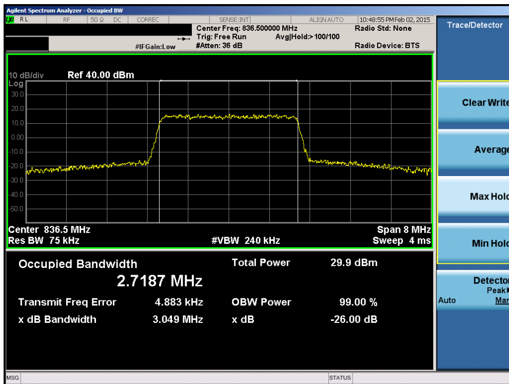
Plot 6-12. Occupied Bandwidth Plot (Band 26 – 3.0MHz 16-QAM – RB Size 15)
