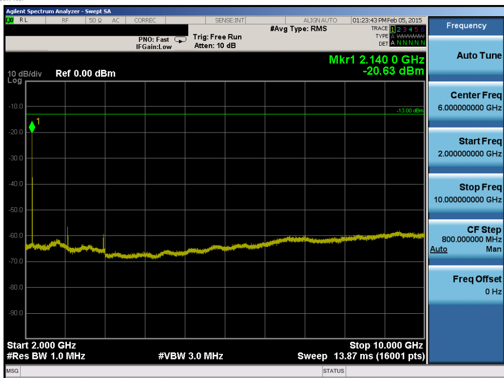
Plot 6-59. Conducted Spurious Plot (Band 12 – 3.0MHz QPSK – RB Size 1, RB Offset 0 – High Channel)
