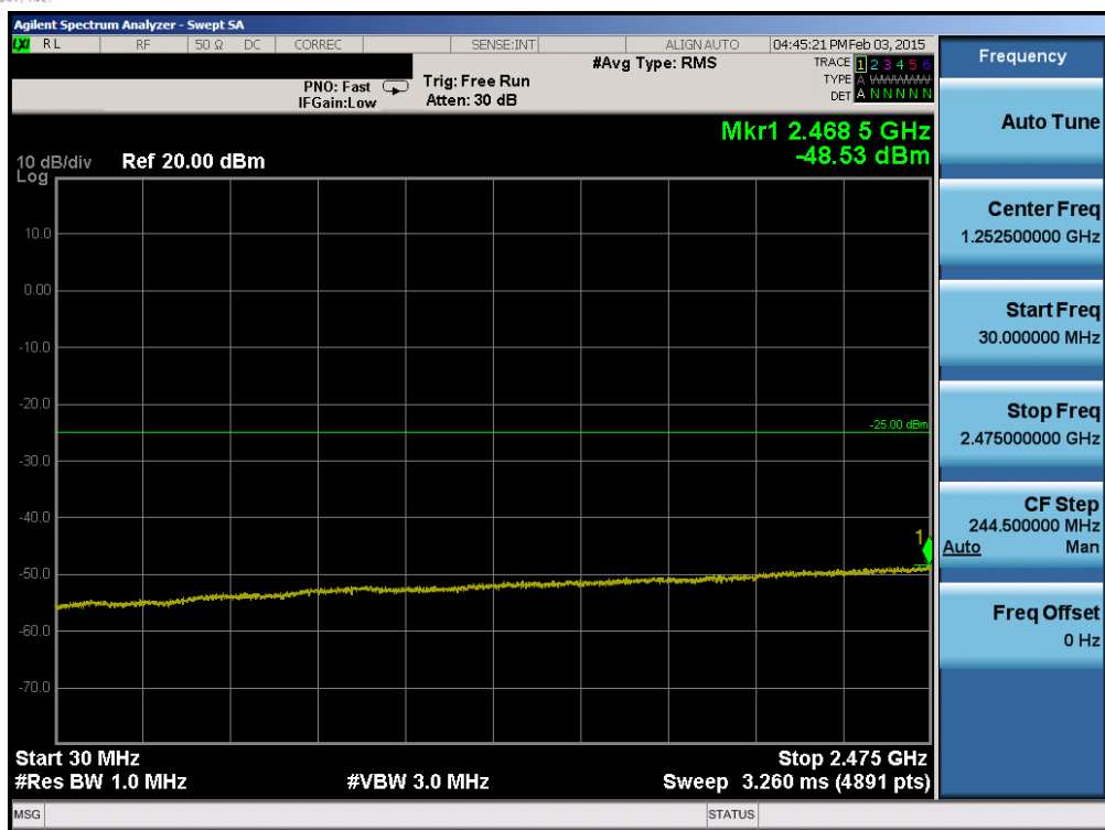
Plot 6-93. Conducted Spurious Plot (Band 41 – 5.0MHz QPSK – RB Size 1, RB Offset 0 – High Channel)
