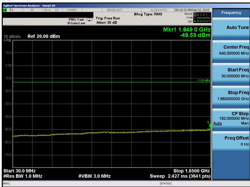
Plot 6-81. Conducted Spurious Plot (Band 25 – 5.0MHz QPSK – RB Size 1, RB Offset 0 – Mid Channel)
