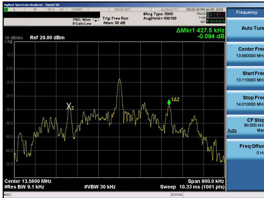
Figure 7-2. 20dB Bandwidth Plot
