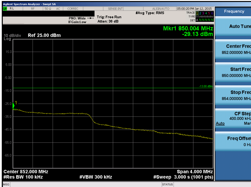
Plot 6-58. Upper Extended Band Edge Plot (Band 26 – Band 5 – 3.0MHz QPSK – RB Size 15)
