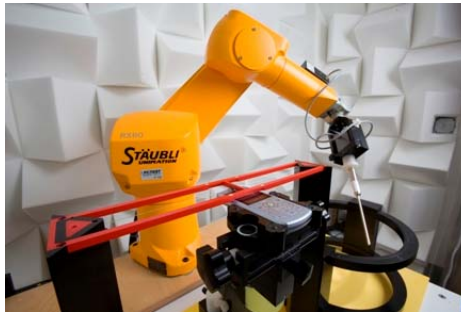
Figure 4-3 SPEAG Robotic System
