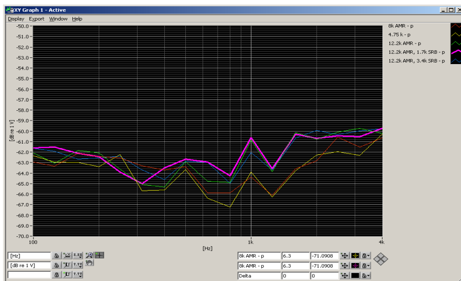
Figure 5-2 UMTS Audio Band Magnetic Noise
