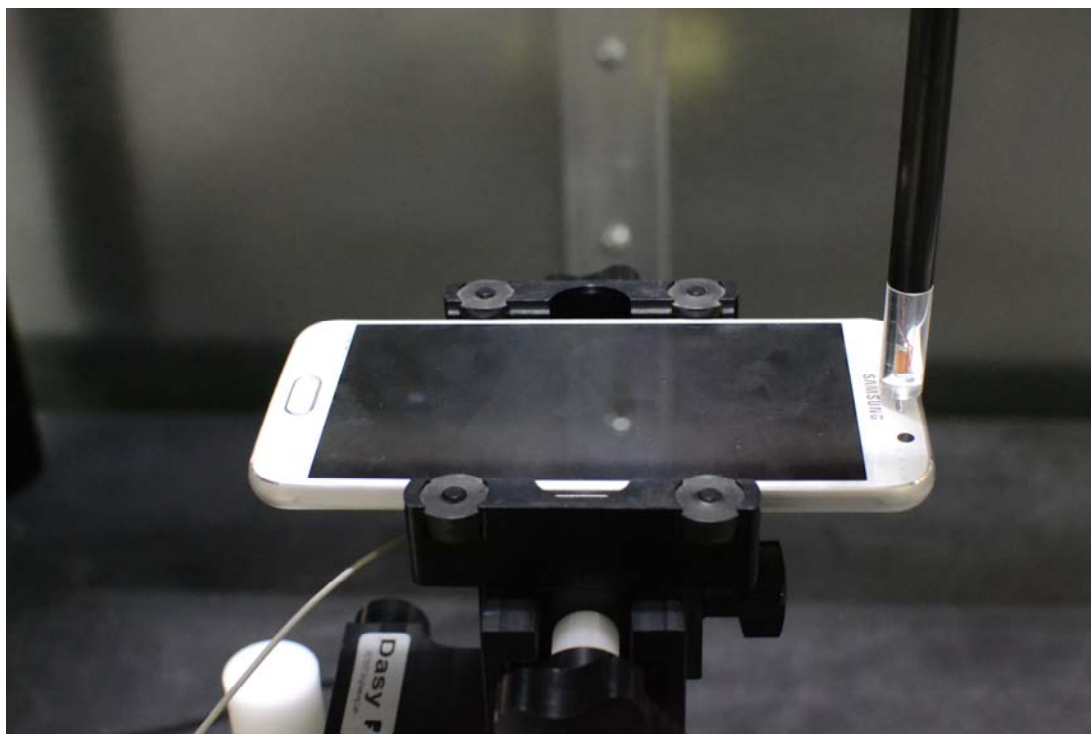
Figure 12-1 Test Setup for Wireless Device
