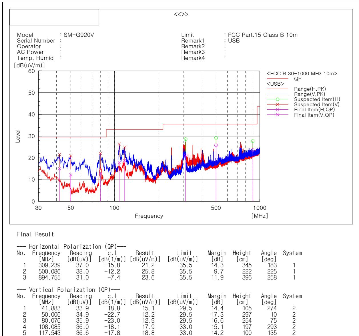
Note) Receiving antenna polarization : Horizontal, Vertical
