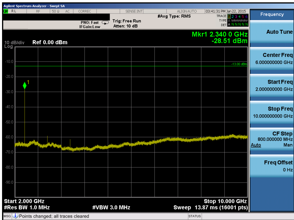
Plot 6-38. Conducted Spurious Plot (Band 13 – 5.0MHz QPSK – RB Size 1, RB Offset 0 – Mid Channel)
