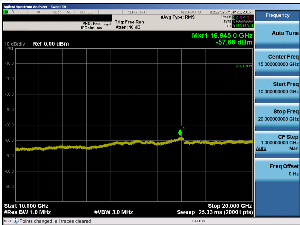
Plot 6-53. Conducted Spurious Plot (Band 4 – 5.0MHz QPSK – RB Size 1, RB Offset 0 – Low Channel)
