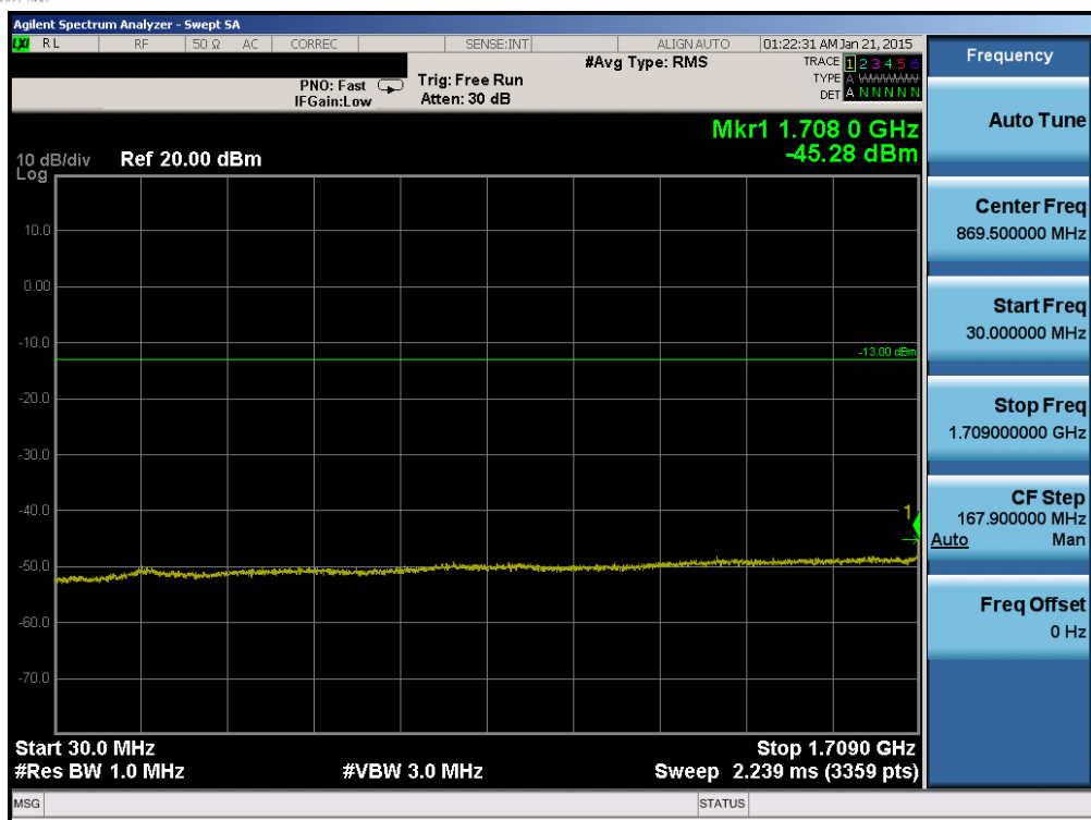
Plot 6-51. Conducted Spurious Plot (Band 4 – 5.0MHz QPSK – RB Size 1, RB Offset 0 – Low Channel)
