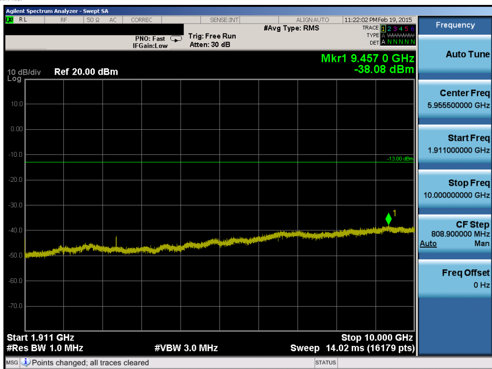
Plot 6-67. Conducted Spurious Plot (Band 2 – 10.0MHz QPSK – RB Size 1, RB Offset 0 – High Channel)
