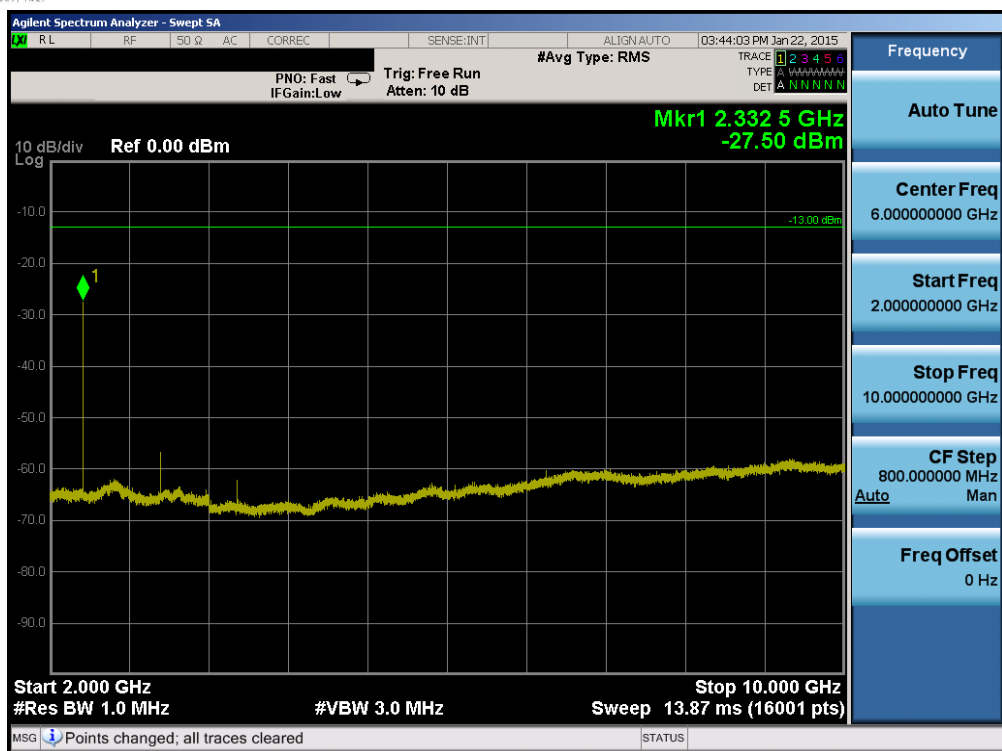
Plot 6-35. Conducted Spurious Plot (Band 13 – 5.0MHz QPSK – RB Size 1, RB Offset 0 – Low Channel)
