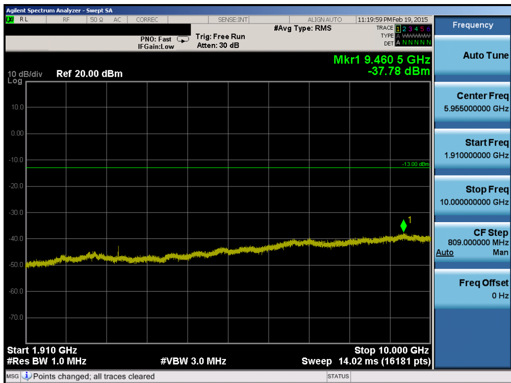
Plot 6-64. Conducted Spurious Plot (Band 2 – 10.0MHz QPSK – RB Size 1, RB Offset 0 – Mid Channel)
