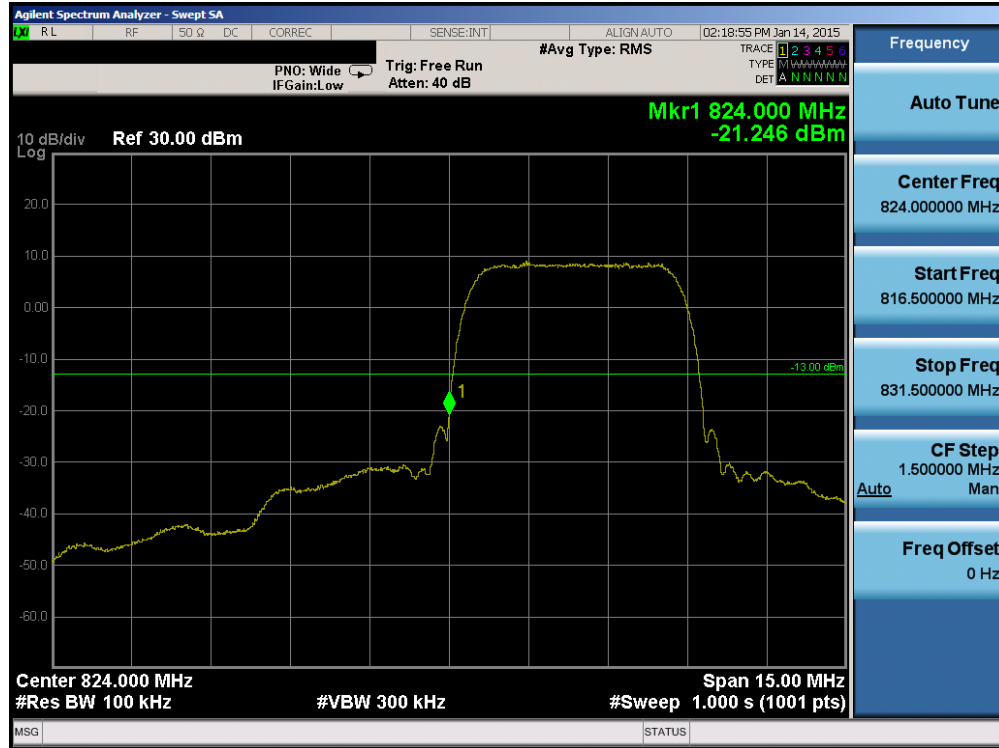
Plot 6-79. Band Edge Plot (Cellular WCDMA Mode – Ch. 4132)
