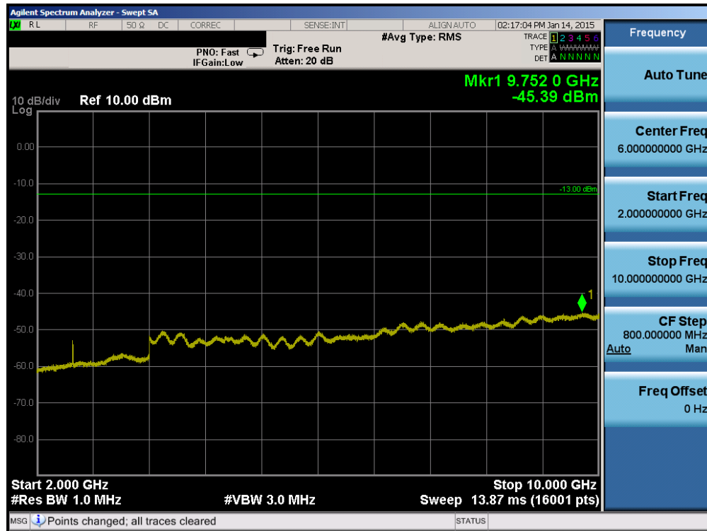
Plot 6-50. Conducted Spurious Plot (Cellular WCDMA Mode – Ch. 4183)
