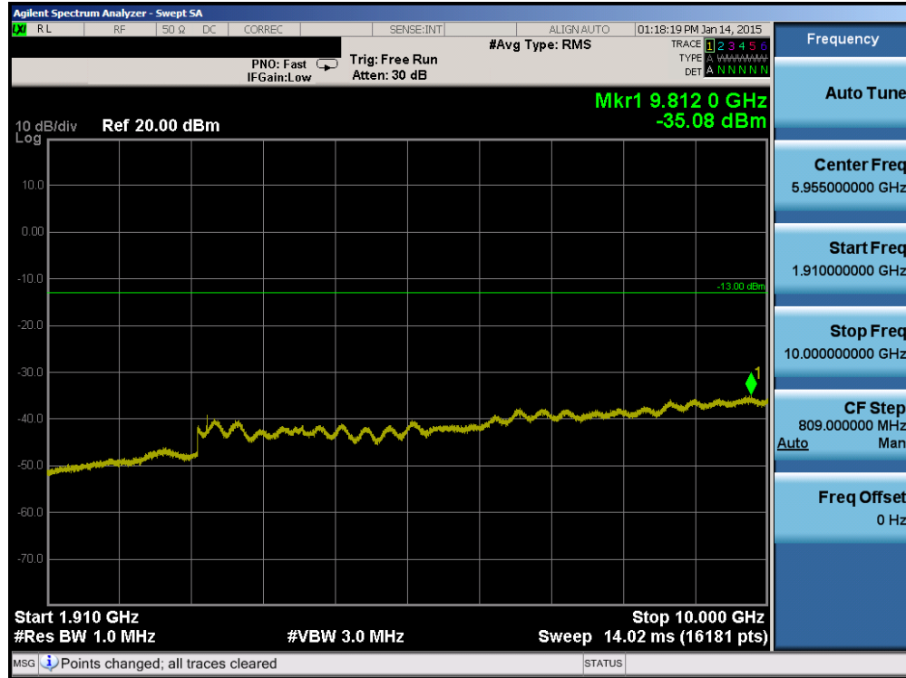
Plot 6-37. Conducted Spurious Plot (PCS CDMA Mode – Ch. 25)
