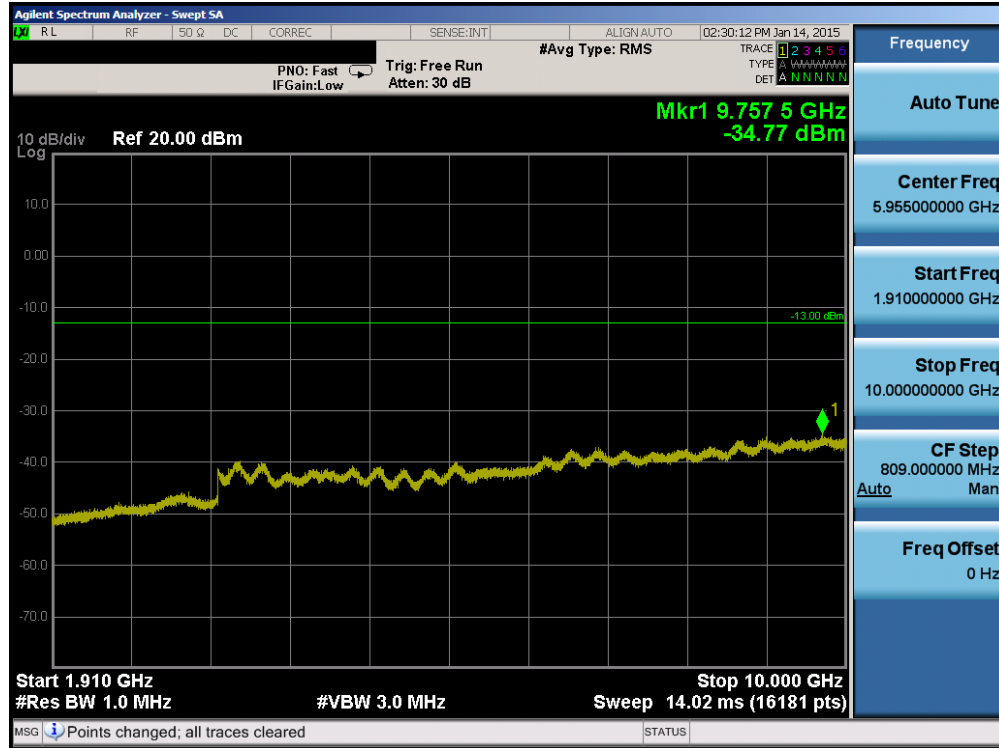
Plot 6-55. Conducted Spurious Plot (PCS WCDMA Mode – Ch. 9262)
