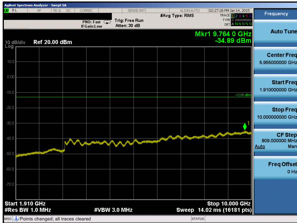
Plot 6-58. Conducted Spurious Plot (PCS WCDMA Mode – Ch. 9400)
