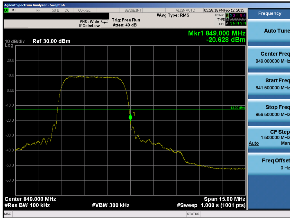
Plot 6-80. Band Edge Plot (Cellular WCDMA Mode – Ch. 4233)
