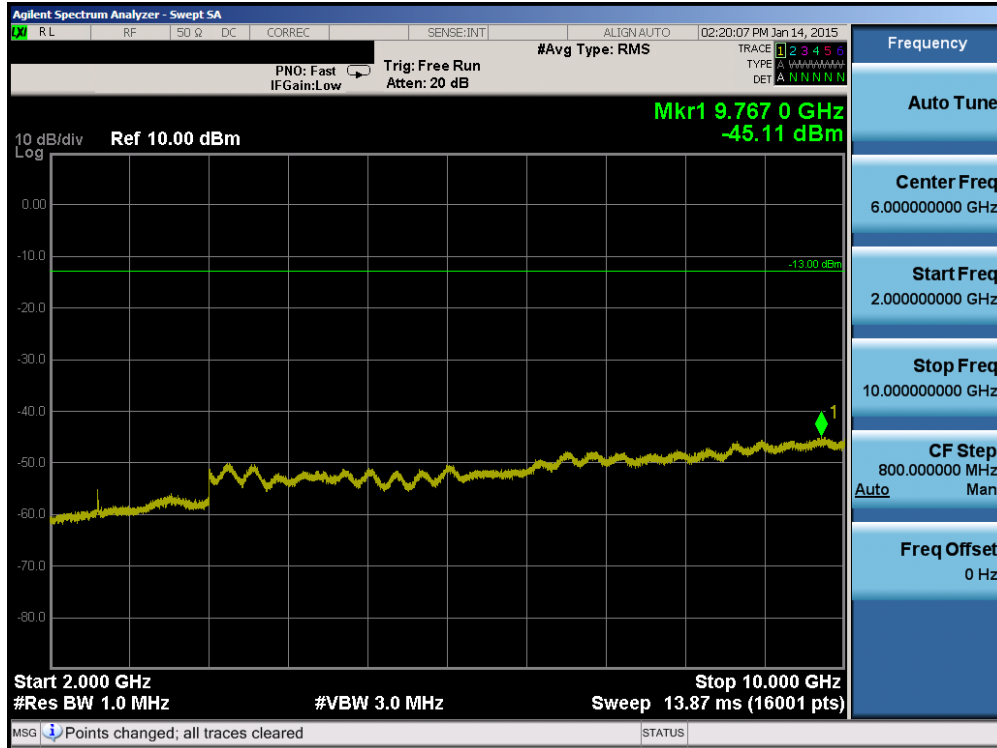
Plot 6-47. Conducted Spurious Plot (Cellular WCDMA Mode – Ch. 4132)
