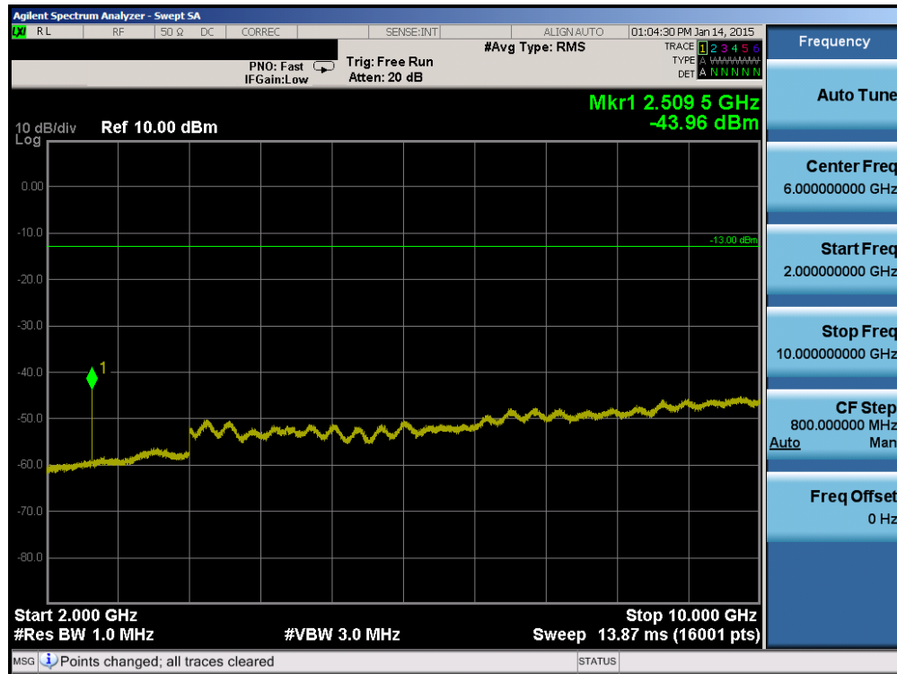
Plot 6-32. Conducted Spurious Plot (Cellular CDMA Mode – Ch. 384)
