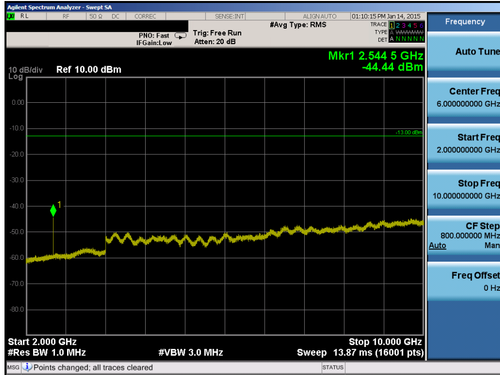
Plot 6-35. Conducted Spurious Plot (Cellular CDMA Mode – Ch. 777)
