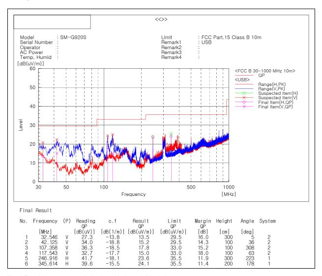
Note) Receiving antenna polarization: Horizontal, Vertical
