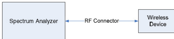
Figure 6-1. Test Instrument & Measurement Setup
