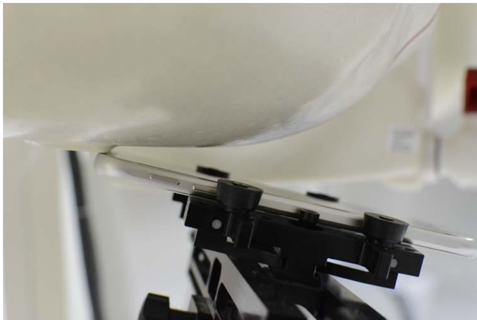
SAR Test Setup Photo 2: Right Tilt
