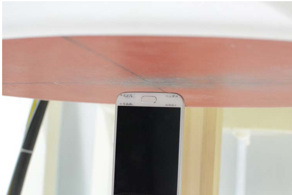
SAR Test Setup Photo 8: Bottom at 1.0 cm
