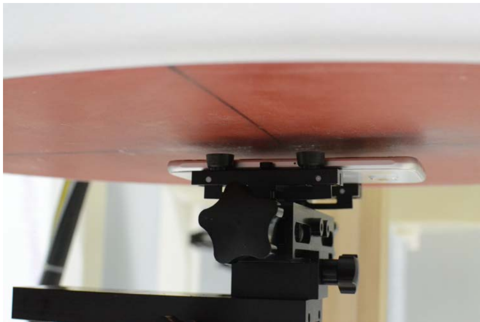
SAR Test Setup Photo 6: Front at 1.0 cm
