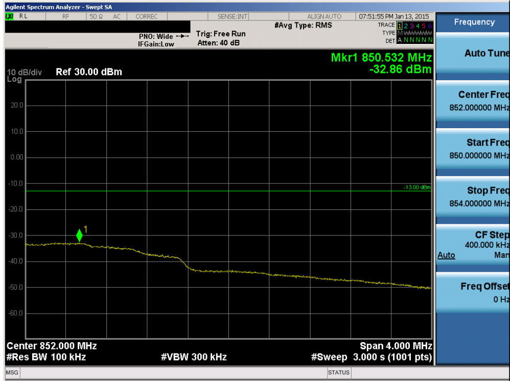
Plot 6-78. Upper Extended Band Edge Plot (Band 26 – Band 5 – 3.0MHz QPSK – RB Size 15)
