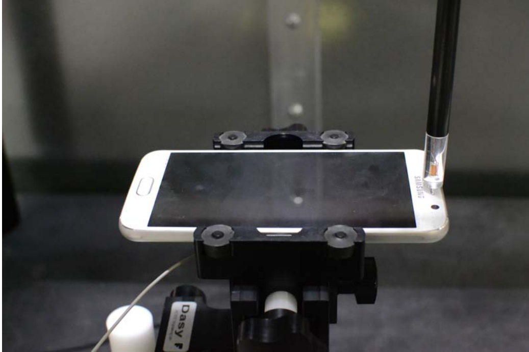
Figure 12-1 Test Setup for Wireless Device
