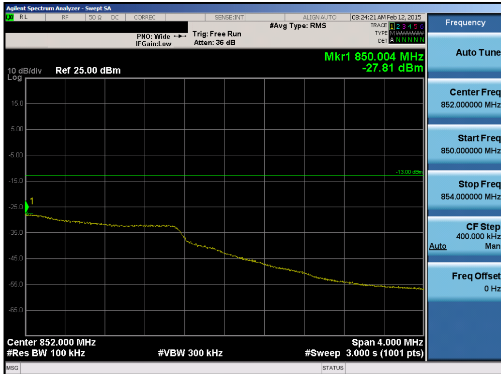
Plot 6-100. Upper Extended Band Edge Plot (Band 26 – Band 5 – 3.0MHz QPSK – RB Size 15)
