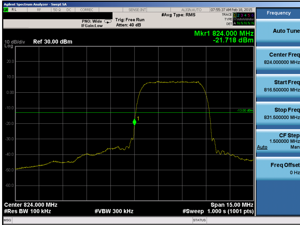
Plot 6-59. Band Edge Plot (Cellular WCDMA Mode – Ch. 4132)
