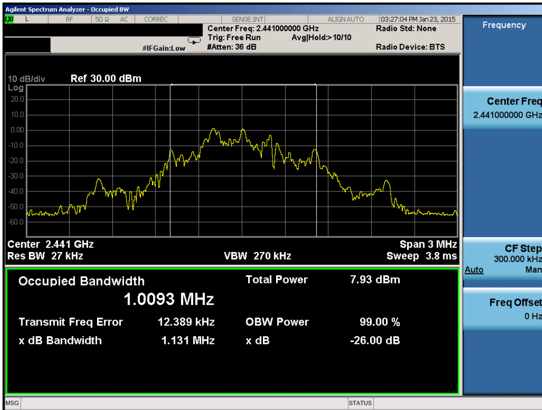
Plot 6-1. Occupied Bandwidth Plot (ANT+ – Ch. 39)
