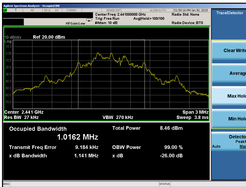
Plot 6-1. Occupied Bandwidth Plot (ANT+ – Ch. 39)
