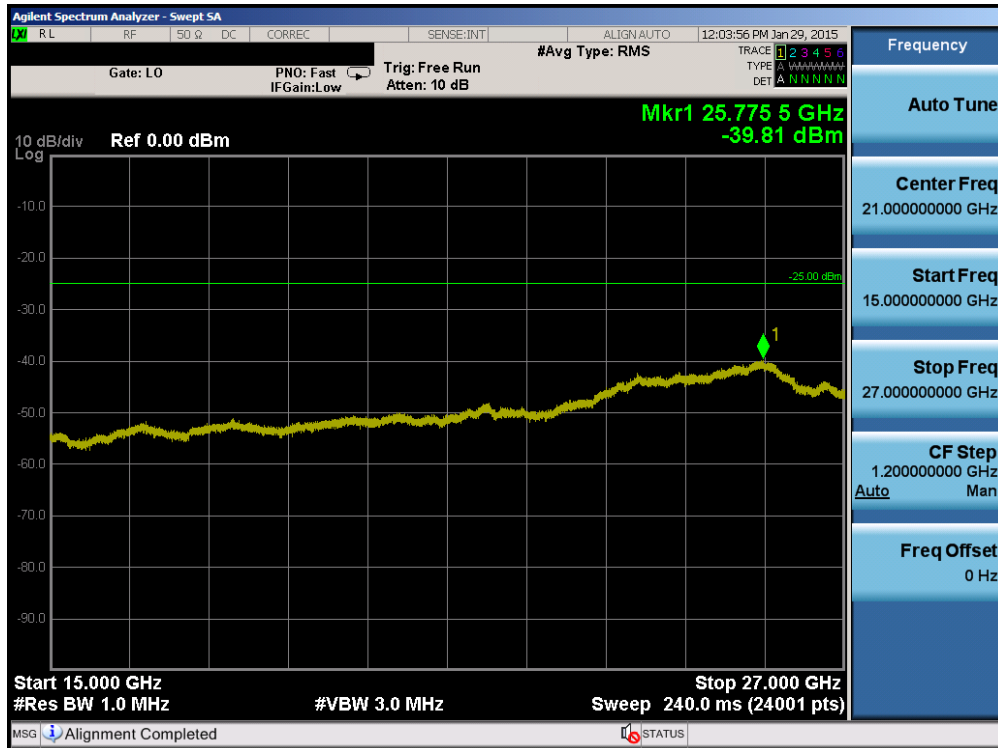
Plot 6-32. Conducted Spurious Plot (Band 41 – 10.0MHz QPSK – RB Size 1, RB Offset 0 – Low Channel)
