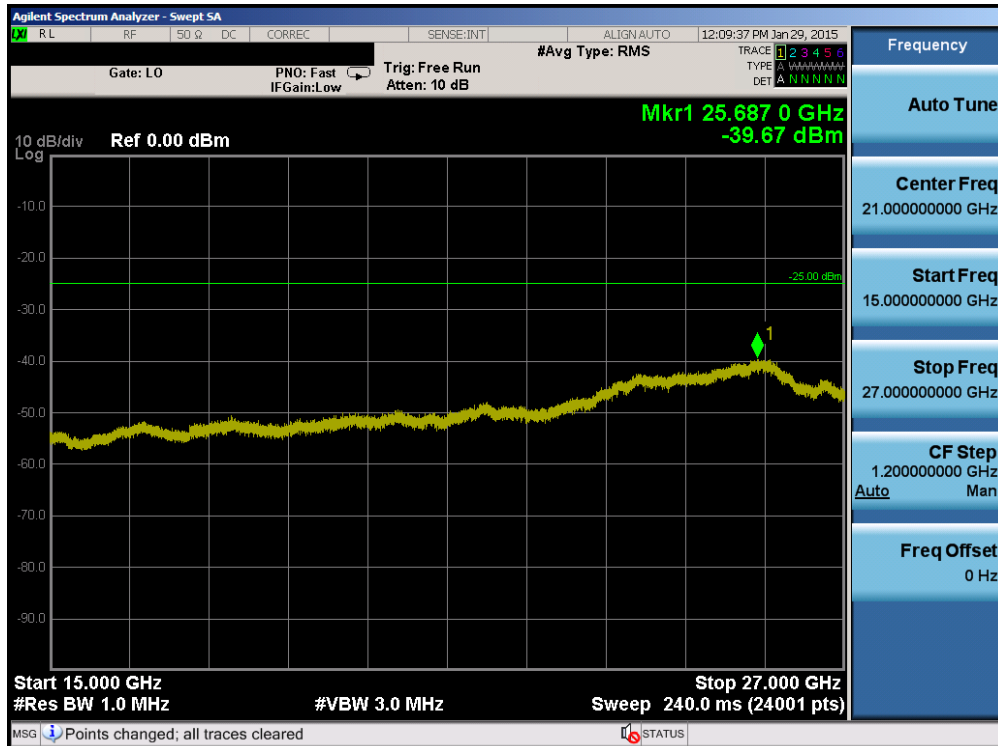
Plot 6-38. Conducted Spurious Plot (Band 41 – 10.0MHz QPSK – RB Size 1, RB Offset 0 – High Channel)
