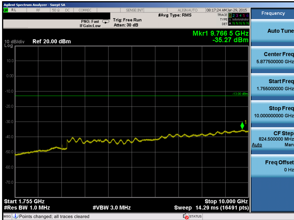
Plot 6-22. Conducted Spurious Plot (Band 4 – 5.0MHz QPSK – RB Size 1, RB Offset 0 – Low Channel)
