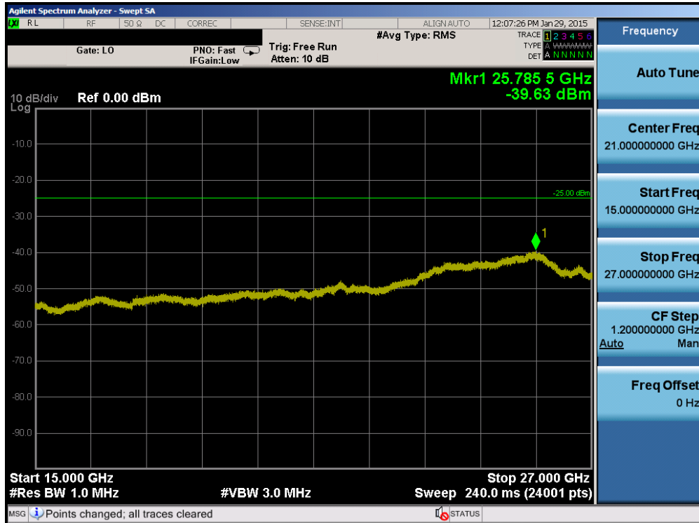
Plot 6-35. Conducted Spurious Plot (Band 41 – 10.0MHz QPSK – RB Size 1, RB Offset 0 – Mid Channel)
