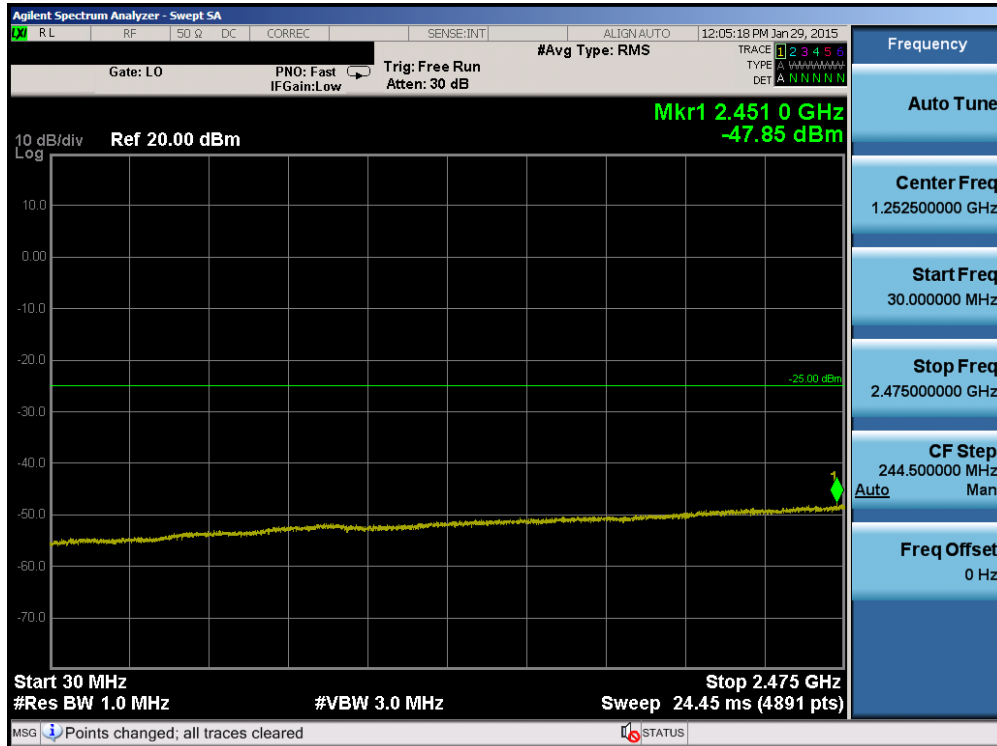
Plot 6-33. Conducted Spurious Plot (Band 41 – 10.0MHz QPSK – RB Size 1, RB Offset 0 – Mid Channel)
