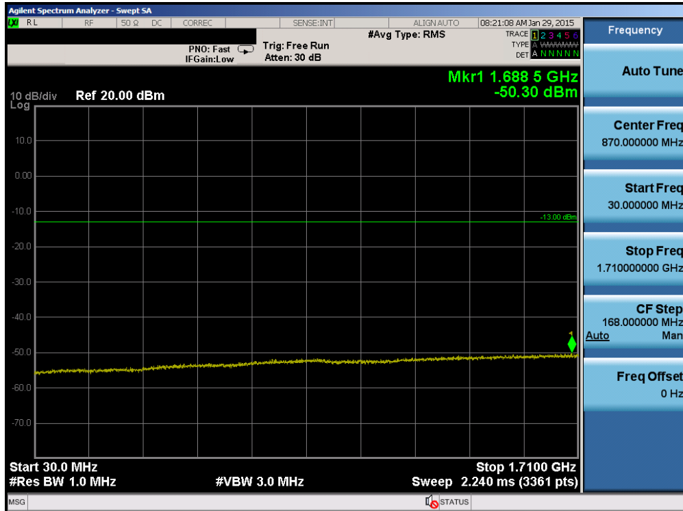
Plot 6-27. Conducted Spurious Plot (Band 4 – 5.0MHz QPSK – RB Size 1, RB Offset 0 – High Channel)
