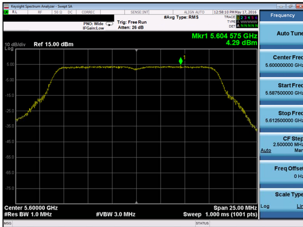
Plot 7-52. Power Spectral Density Plot (802.11a (UNII Band 2C) – Ch. 120)
