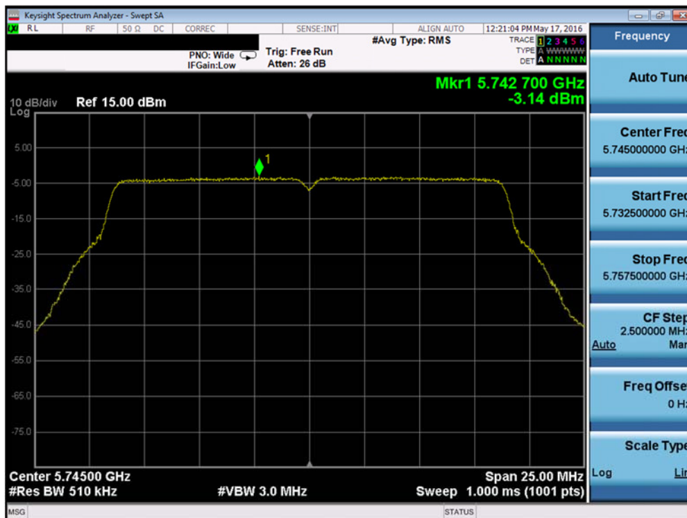
Plot 7-46. Power Spectral Density Plot (20MHz BW 802.11n (UNII Band 3) – Ch. 149)
