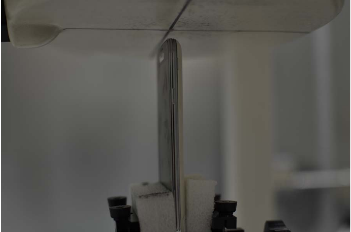
SAR Test Setup Photo 13 – Top Edge, Wireless Charging Cover at 1.0 cm
