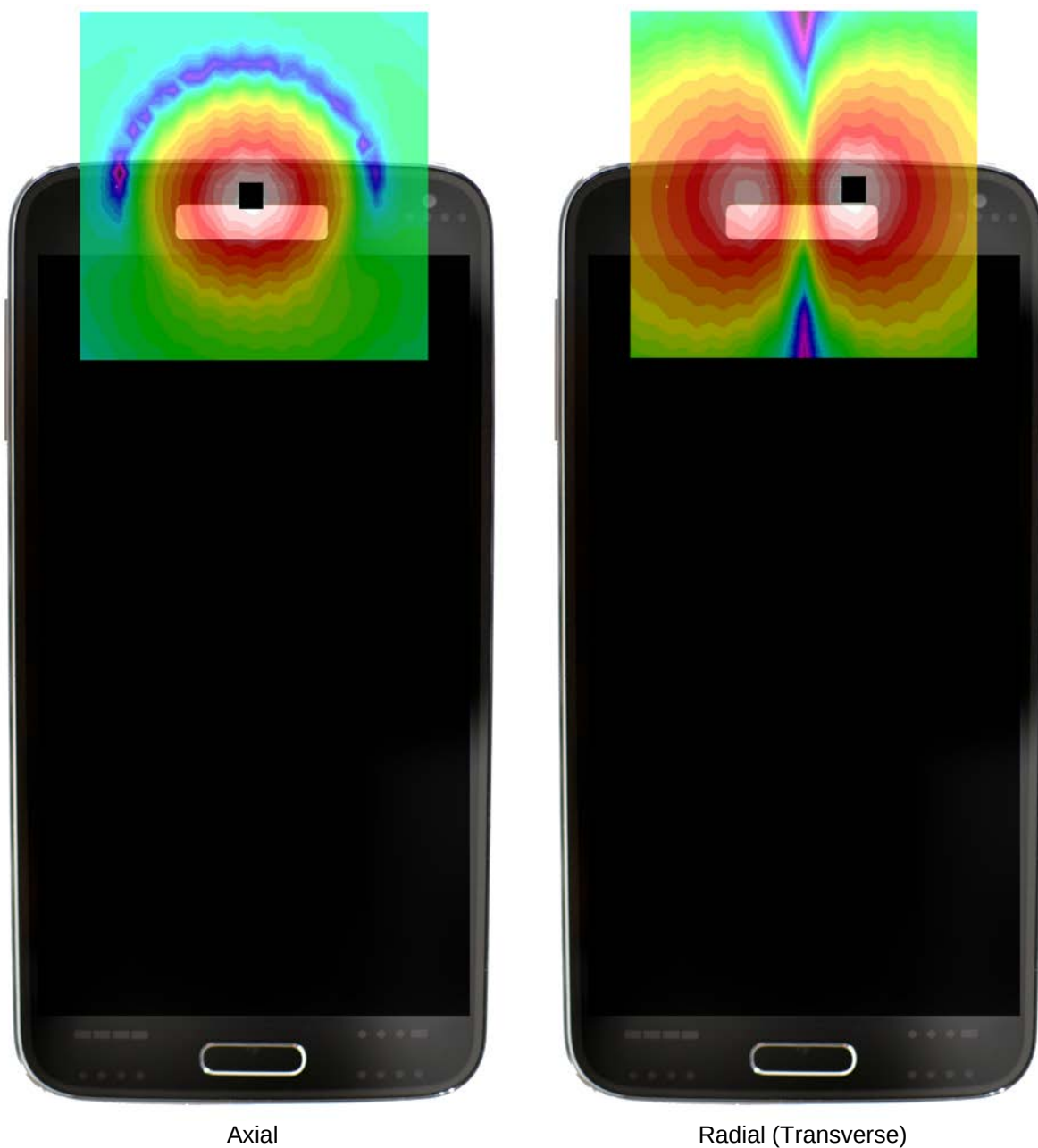
Figure 13-3 T-Coil Scan Overlay Magnetic Field Distributions
