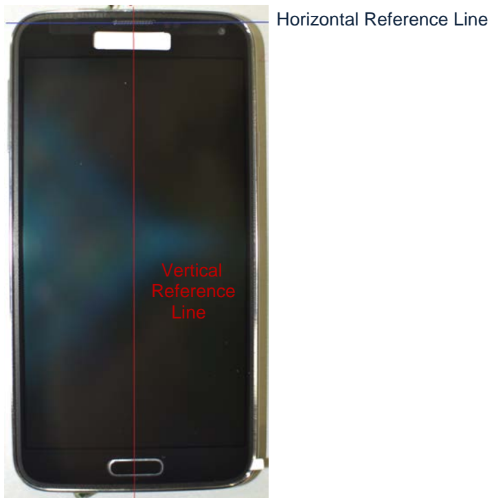
SAR Test Setup Photo 11 – Horizontal and Vertical Reference Lines
