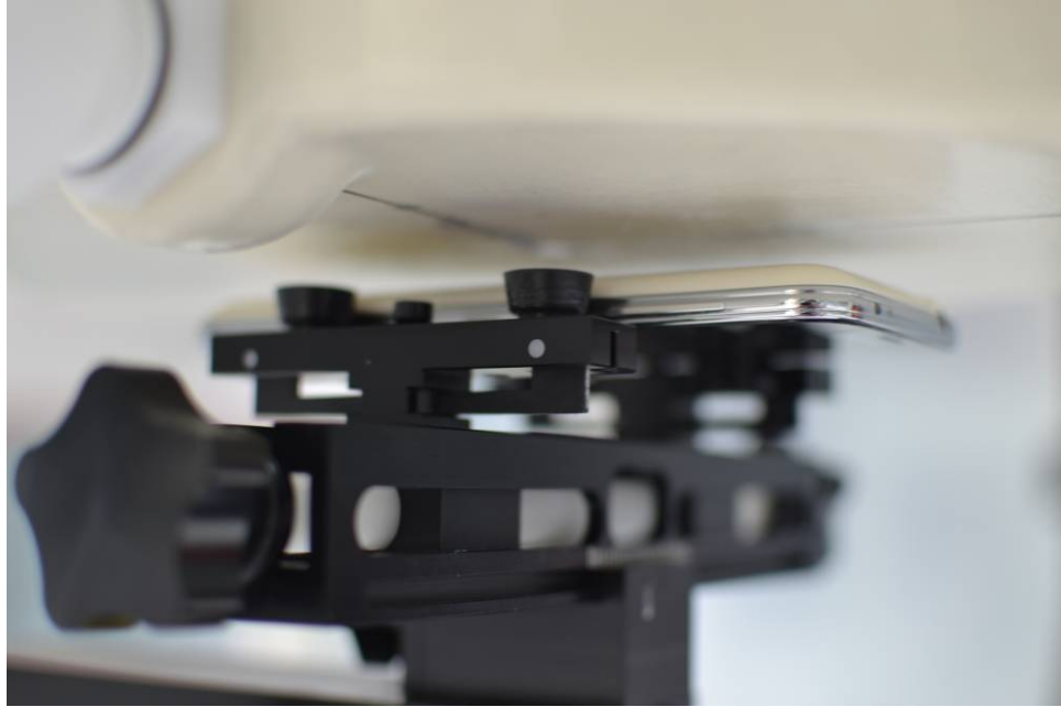
SAR Test Setup Photo 9: Back Side at 1.0 cm with Wireless Charging Cover
