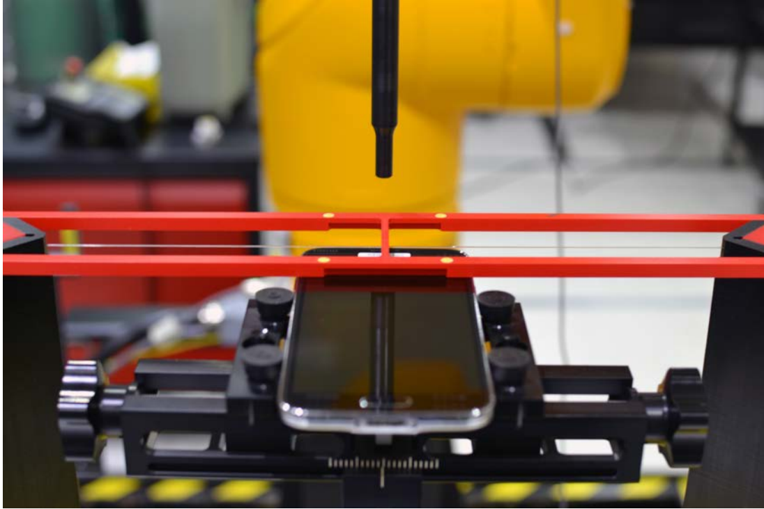
Figure 18-1 Ear Reference Point HAC Phantom Alignment
