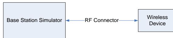
Figure 9-1 Power Measurement Setup
