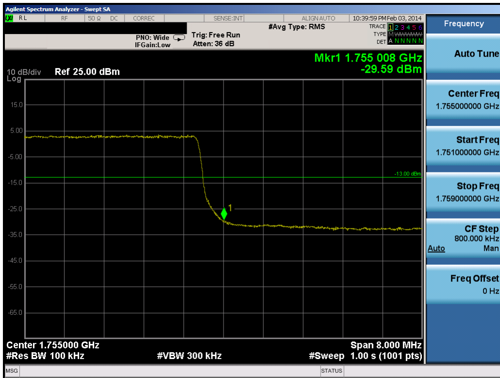
Plot 8-19. Upper Band Edge Plot (10.0MHz QPSK – RB Size 50)
