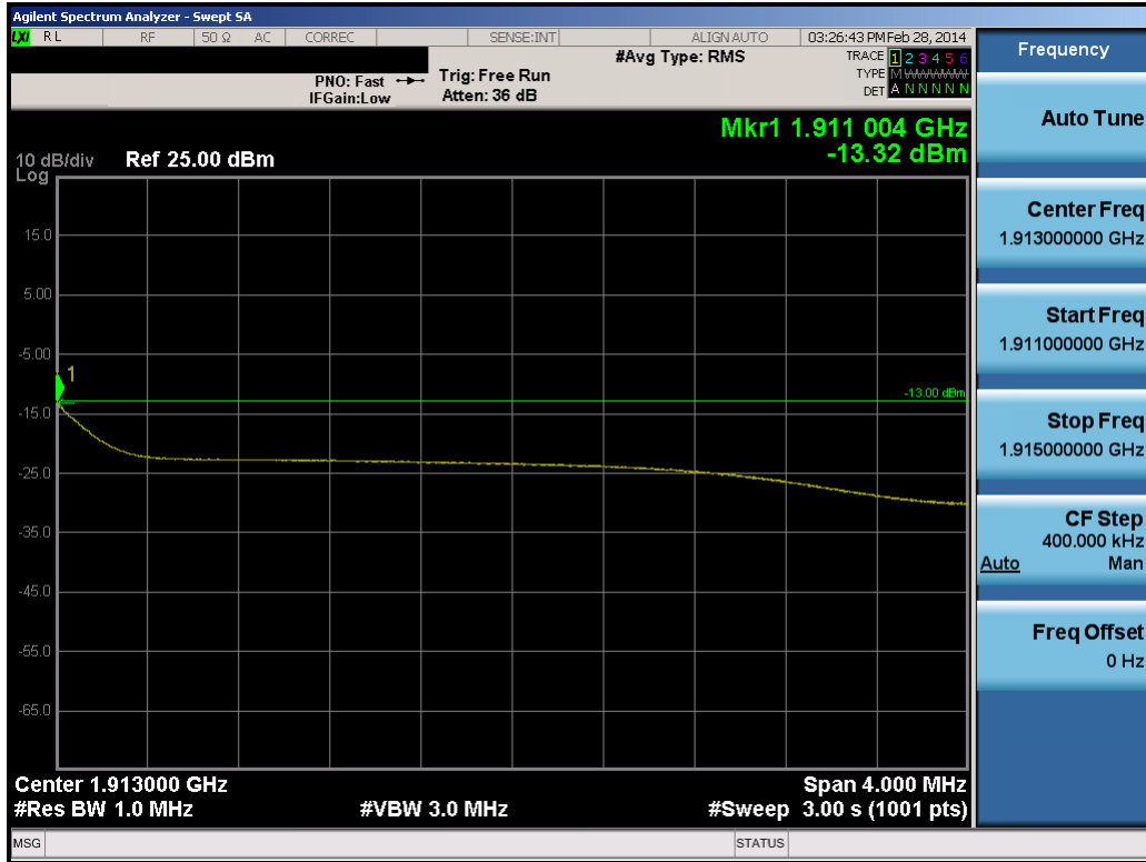
Plot 9-6. Upper Extended Band Edge Plot (5.0MHz QPSK – RB Size 25)
