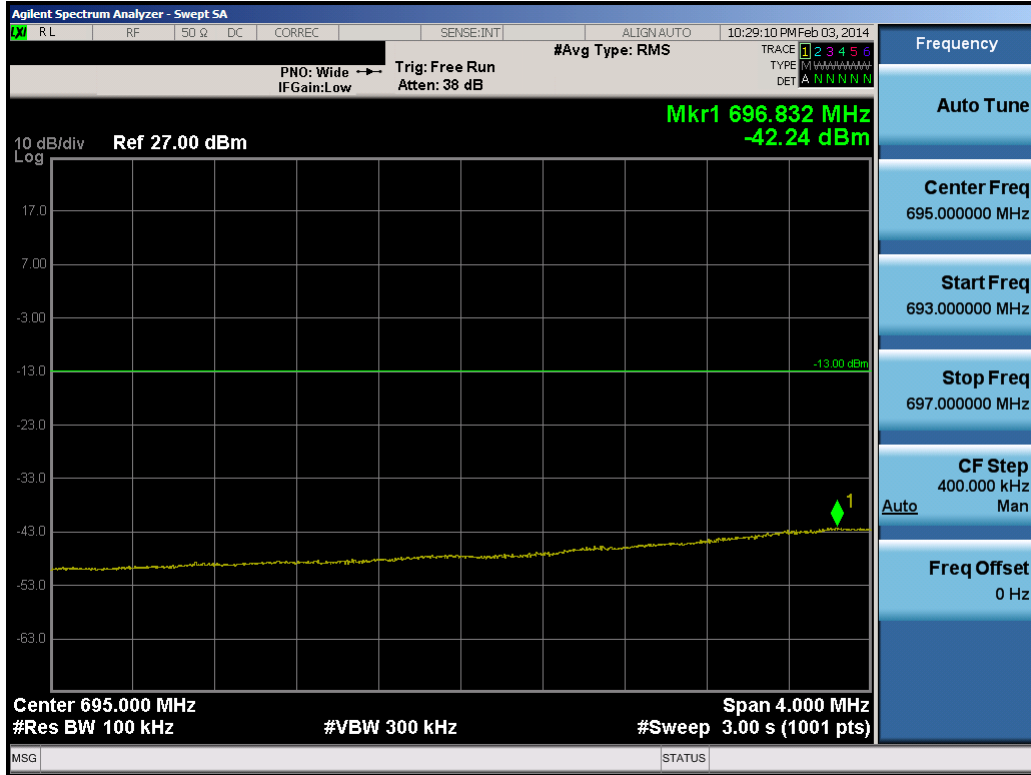
Plot 7-6. Lower Extended Band Edge Plot (10.0MHz QPSK – RB Size 50)
